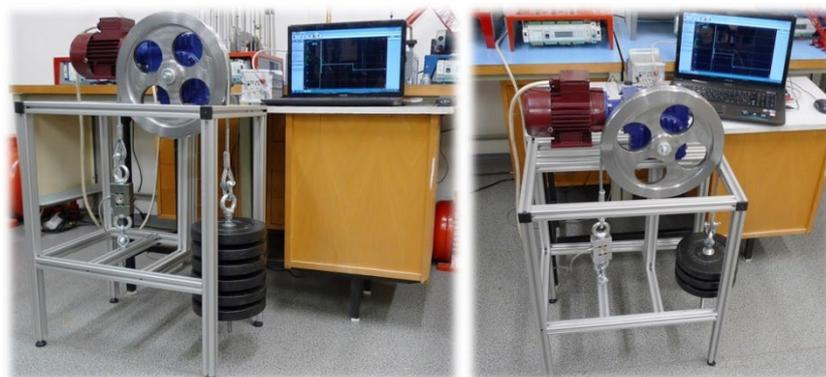
**Figure 17.** Implementation of a laboratory device used to measure tensile forces in the side of a rope approaching the rope sheave.
