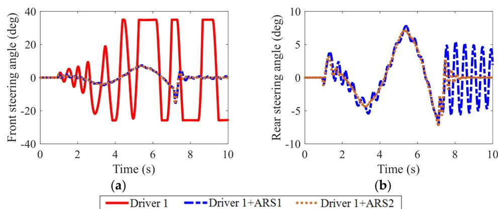
**Figure 11.** Front and rear steering angles of vehicles in Case B: (a) front steering angle; (b) rear steering angle.
