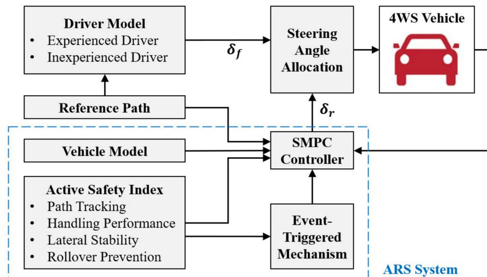
**Figure 1.** Control system framework of human driver and ARS system.
