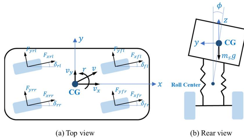
Figure 3. 4WS vehicle dynamic model.
