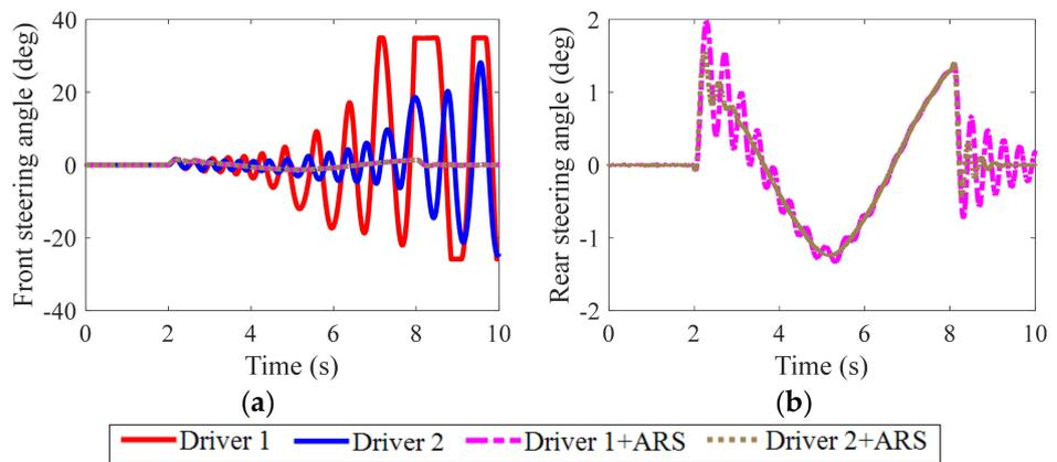
**Figure 7.** Front and rear steering angles of vehicles in Case A: (a) front steering angle; (b) rear steering angle.
