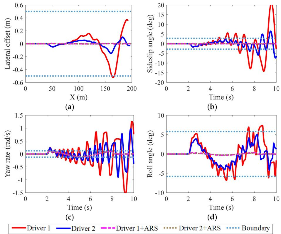
**Figure 6.** Active safety performances of vehicles in Case A: (a) lateral offset; (b) sideslip angle; (c) yaw rate; (d) roll angle.
