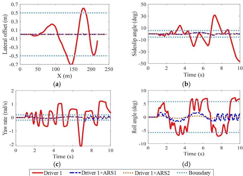
Figure 10. Active safety performances of vehicles in Case B: (a) lateral offset; (b) sideslip angle; (c) yaw rate; (d) roll angle.
