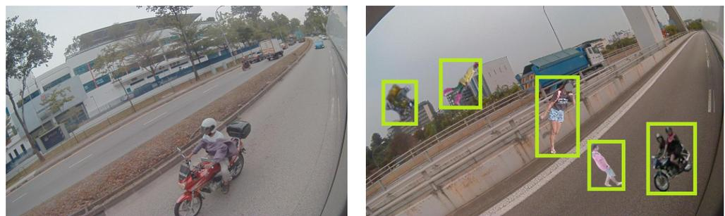
**Figure 6.** (Left) Sample image from side camera, showing the unconventional viewing angle of objects not found in public datasets. (Right) Generated image with objects and their bounding boxes imposed on a random scene.
