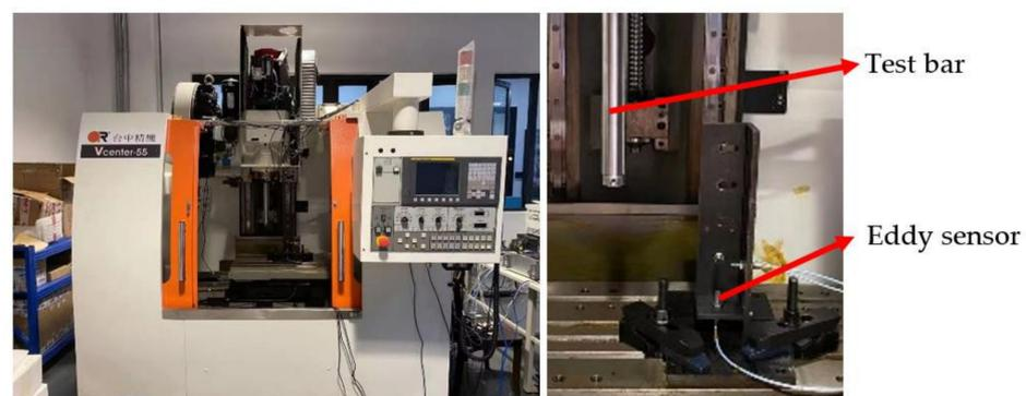
Figure 3. Thermal-error-measurement experiment.
