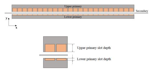
Figure 1. Double-sided LIM with asymmetric primaries (ADSLIM).
