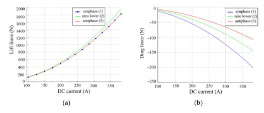
**Figure 7.** Lift force (a) and drag force (b) of ADSLIM in DC mode for three configurations of the magnetic field shown in Figure 6.
