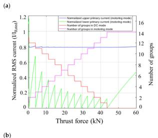
**Figure 12.** Operation diagram of the system for different thrust forces with a weight variation of  $\pm 20\%$ : (a) lift force of 78.5 kN (vehicle weight 8000 kg), (b) lift force of 117.7 kN (vehicle weight 12,000 kg).
