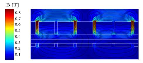
Figure 5. Magnetic field distribution for rated operating conditions.
