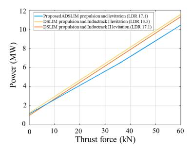
**Figure 13.** Power consumption comparison of the proposed ADSLIM-based system and equivalent passive PM-based maglev systems "DSLIM Inductrack I" and "DSLIM Inductrack II"; constant lift force of 98.1 kN is assumed in all cases.
