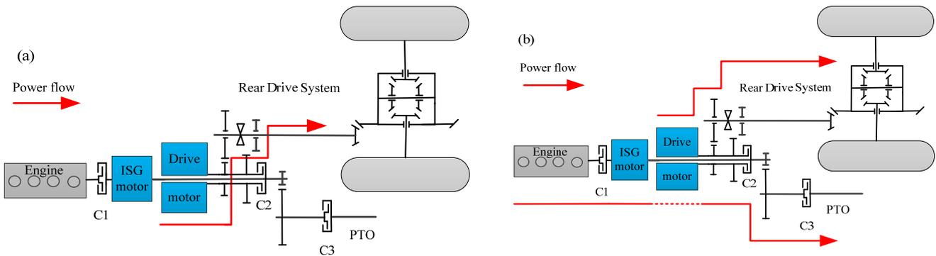
Figure 2. Power flow in SM1 (a) and SM2 (b) modes.
