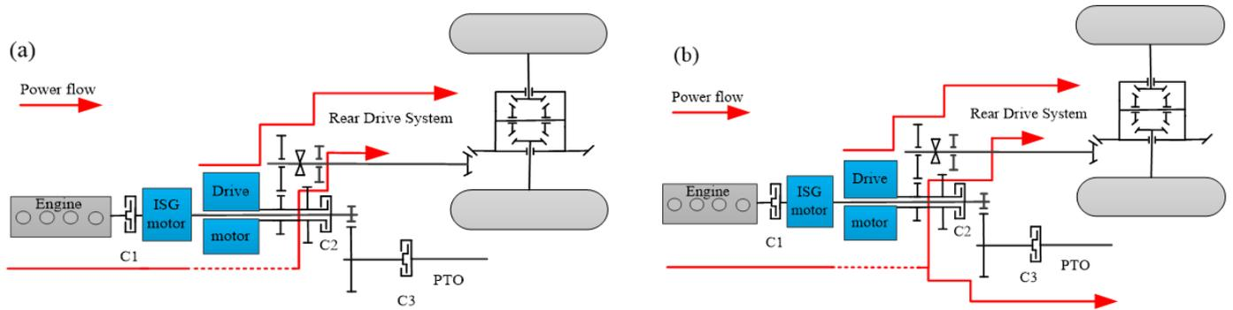
Figure 3. Power flow in TC (a) and STC (b) modes.
