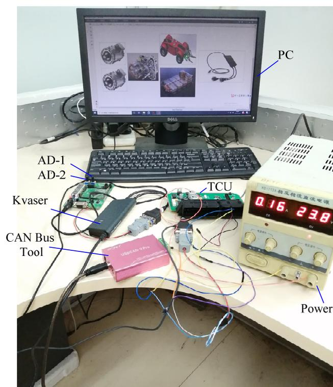
**Figure 9.** Hardware-in-loop test bench.
