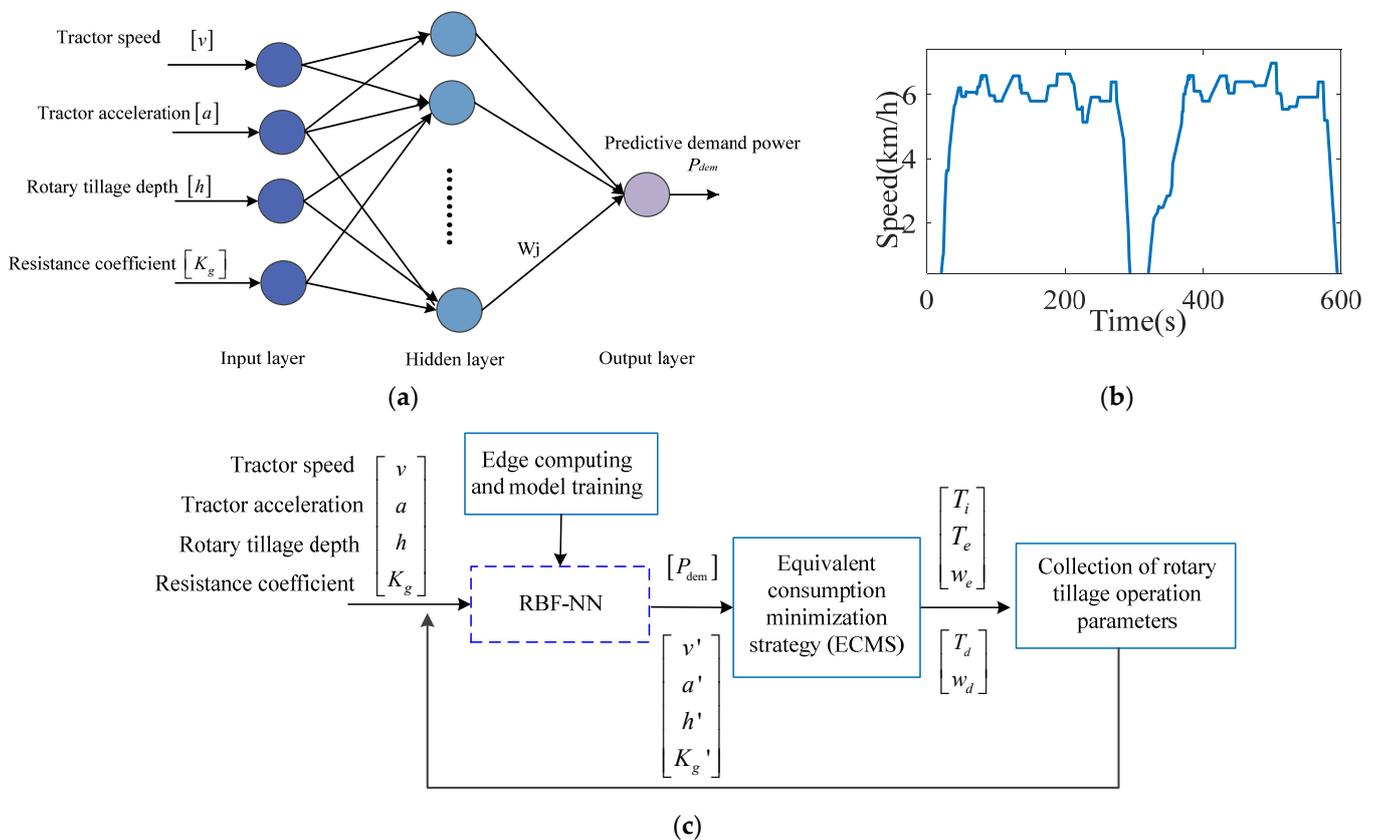
**Figure 5.** The scheme of equivalent consumption minimization strategy. (a) The structure of RBF neural network. (b) The speed curve of tractor rotary tillage. (c) ECMS based on predictive power demand.
