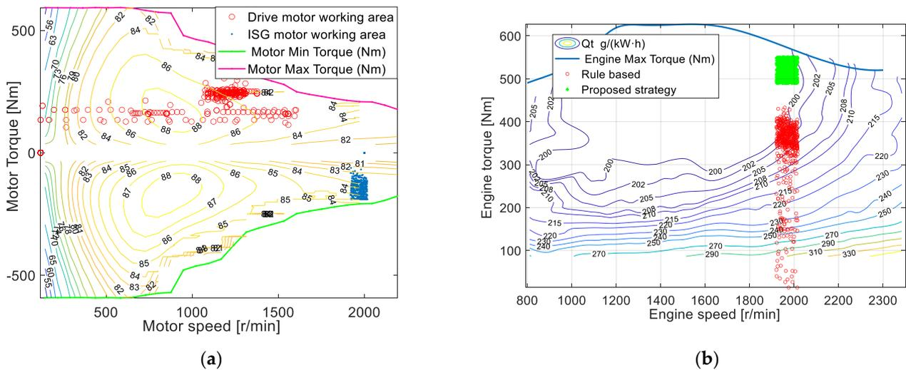
**Figure 10.** The working area of power units. (a) The working area of motors in rotary tillage. (b) The working area of the engine in rotary tillage.
