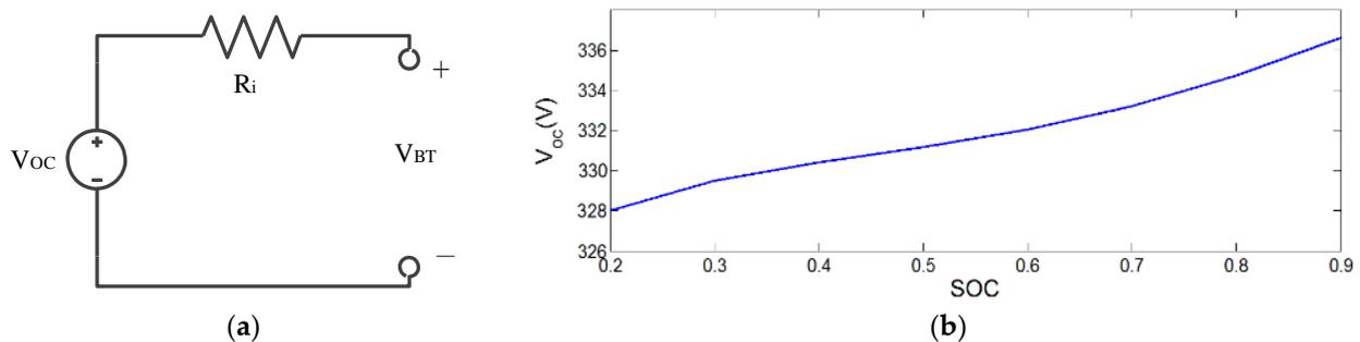
**Figure 4.** Model of the battery pack. (a) The battery diagram of the equivalent circuit. (b) The correlation between the battery open-circuit voltage and SOC.
