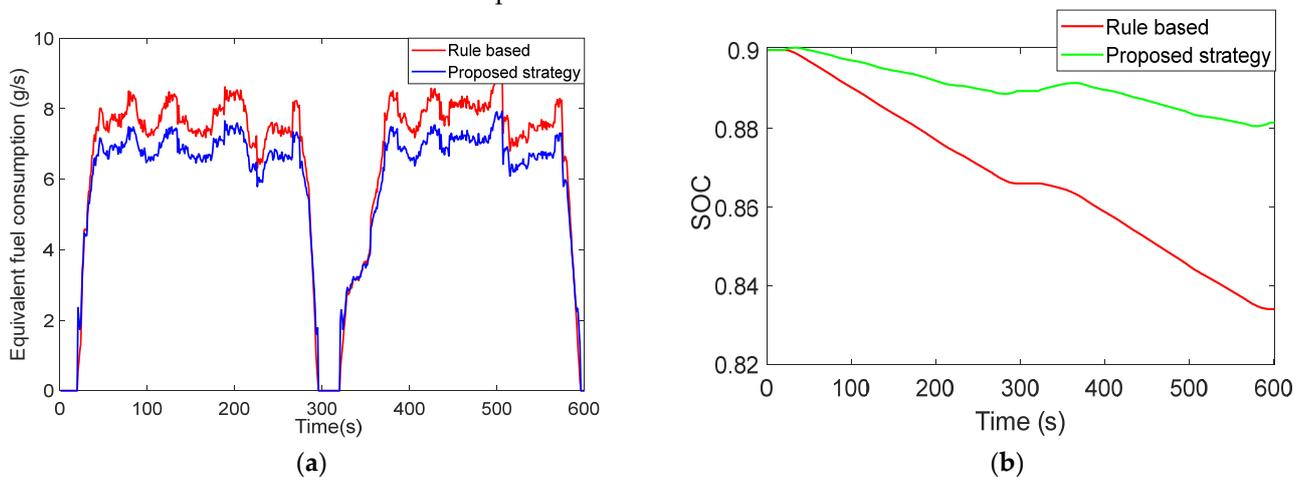
**Figure 11.** The results of the proposed strategy. (a) The optimized equivalent fuel consumption. (b) The SOC curve of battery in rotary tillage conditions.
