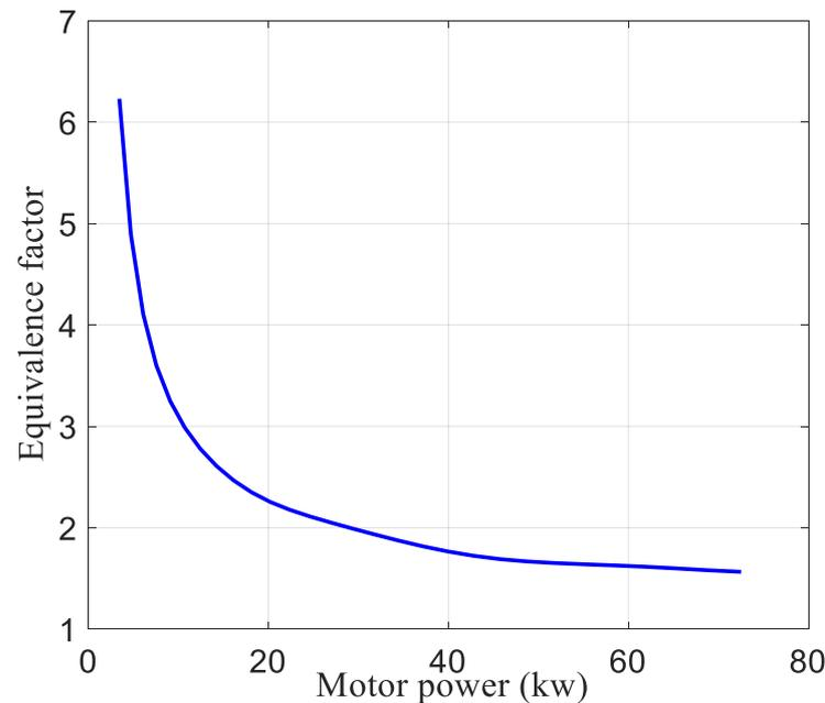
**Figure 6.** The fitting curve between motor power and equivalence factor.
