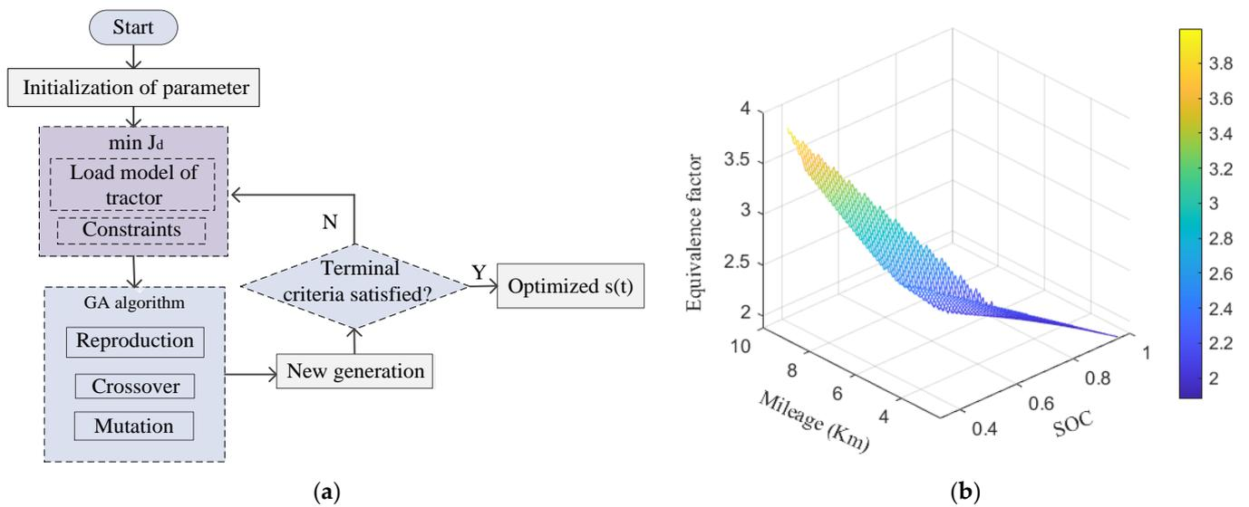
**Figure 7.** The optimized equivalence factor. (a) The process of GA optimization. (b) Equivalent factors under different SOC and rotary tillage mileages.
