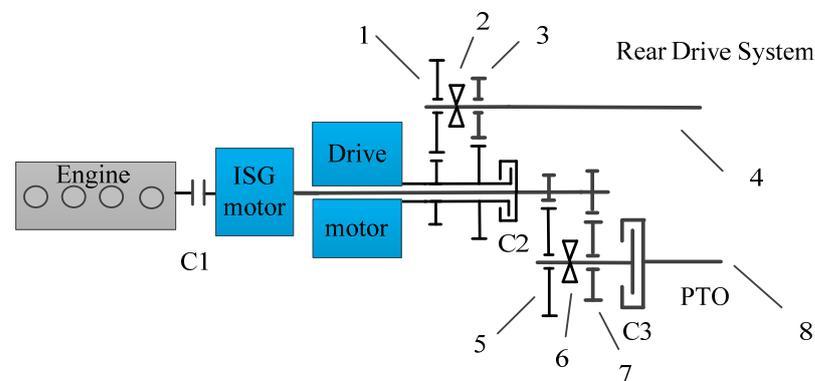
**Figure 1.** The configuration of the coupled-split power system. (1) Low gear; (2) synchronizer; (3) high gear; (4) rear driveshaft; (5) low gear of PTO; (6) synchronizer; (7) intermediate gear of PTO; (8) PTO.
