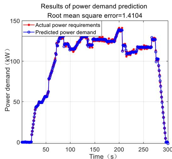
**Figure 8.** Power demand forecasting based on RBF-NN.
