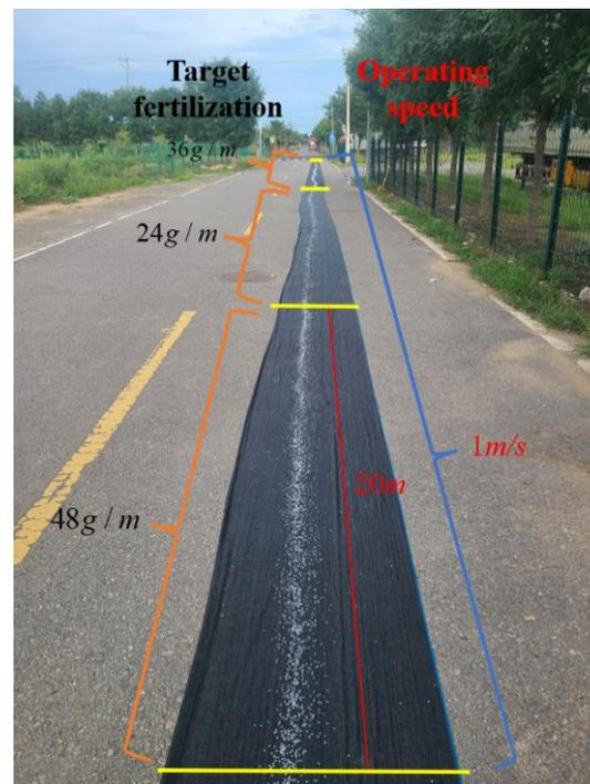
Figure 16. Precision test of fertilizer discharge under different amounts.
