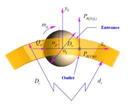
Figure 8. Forces between the *j*th ball and the cage.
