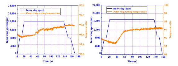
Figure 25. Experimental results for the temperature of the outer ring under 16,000 rpm and 17,000 rpm.
