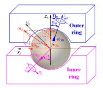
Figure 6. The motion of the ball.
