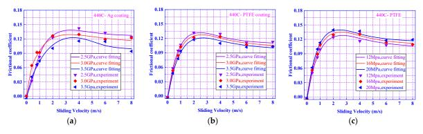
**Figure 4.** The comparisons between the computation results and the experimental data. (**a**) 440C-Ag coating. (**b**) 440C-PTFE coating. (**c**) 440C-solid PTFE.
