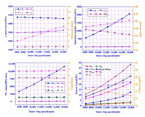
**Figure 20.** Influence of bearing speed  $n_i$  on power loss.
