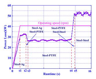
Figure 11. Power loss of ball bearing during the operation.
