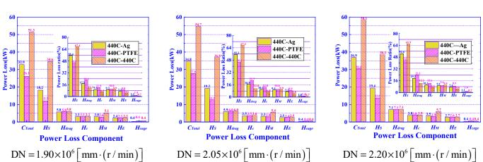
When the ball bearing is working at different speeds, the components of power loss in the three stages are shown in Figure 12.
