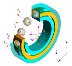
Figure 5. Coordinate systems of the ball bearings.
