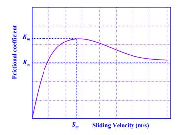
Figure 2. Change of frictional coefficient with sliding velocity [35].
