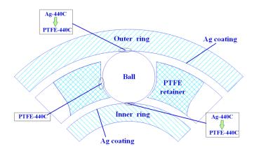
Figure 1. The lubrication states of bearing contact surfaces in the different working stages.
