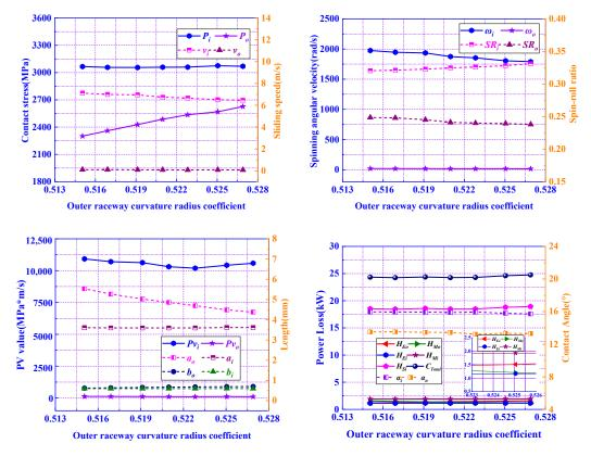
**Figure 17.** Influence of outer raceway curvature radius coefficient  $f_0$  on power loss.
