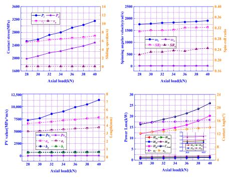
**Figure 18.** Influence of axial load *F*<sub>a</sub> on power loss.
