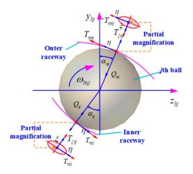
Figure 7. Forces between the *j*th ball and the raceways.
