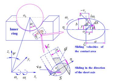
Figure 10. Sliding velocities of the area d*S* in the elliptical contact area.
