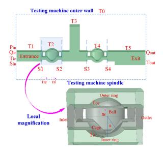
Figure 22. A coupled fluid-thermal finite element model.
