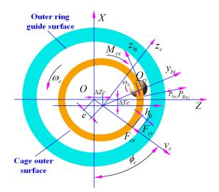
Figure 9. Forces acting on the cage.
