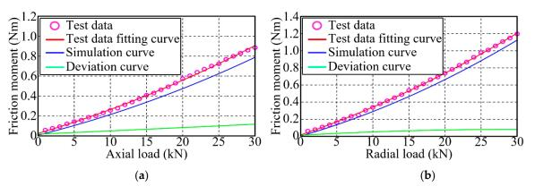
**Figure 12.** Effect of load on friction torque. (**a**) Effect of axial load on friction torque. (**b**) Effect of radial load on friction torque.
