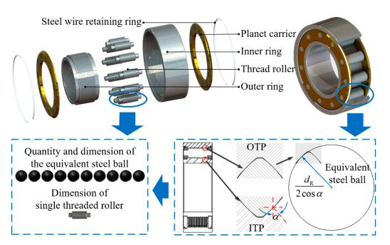
Figure 1. Schematic diagram of PTRB structure composition and equivalent steel ball.
