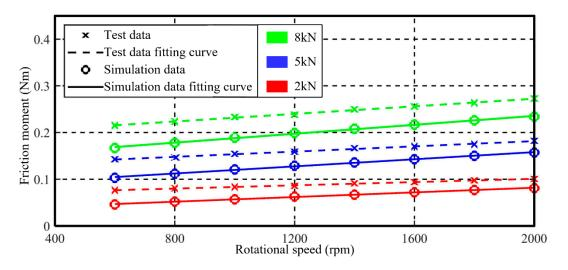
Figure 13. Influence of bearing speed on friction torque under axial load.
