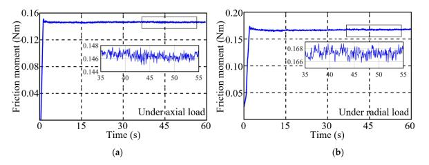
**Figure 11.** Friction torque curve under axial load and radial load. (**a**) Friction torque curve under axial load. (**b**) Friction torque curve under radial load.
