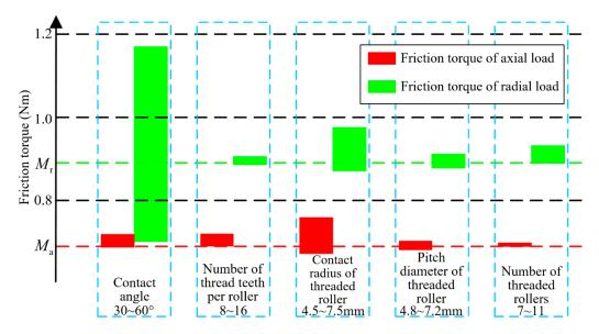
Figure 6. Influence of different structural parameters on friction torque.
