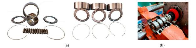
Figure 10. Cleaning and installation of PTRB. (a) Cleaning of PTRB. (b) Installation of PTRB.
