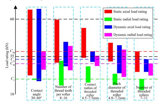
Figure 5. Influence of different structural parameters on load rating.
