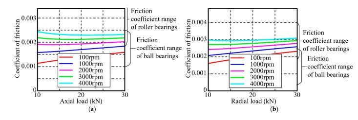
**Figure 4.** Variation of friction coefficient of PTRB prototype with external load and bearing speed. (a) Variation of friction coefficient with axial load and bearing speed. (b) Variation of friction coefficient with radial load and bearing speed.
