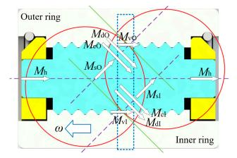
Figure 2. Schematic diagram of each friction torque.
