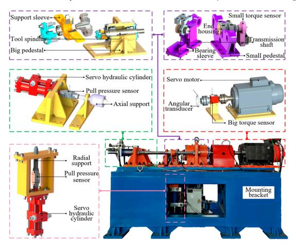
Figure 8. Mechanical scheme of dedicated performance test system.
