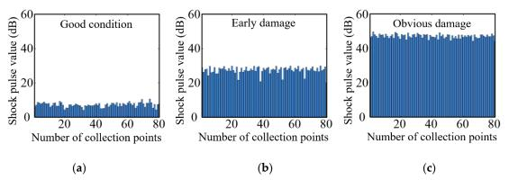
**Figure 15.** Relationship between shock pulse value and bearing health status. (**a**) Good condition. (**b**) Early damage. (**c**) Obvious damage.
