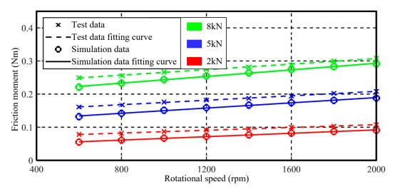
Figure 14. Influence of bearing speed on friction torque under radial load.
