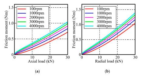
**Figure 3.** Variation of friction torque of PTRB prototype with external load and bearing speed. (a) Variation of friction torque with axial load and bearing speed. (b) Variation of friction torque with radial load and bearing speed.
