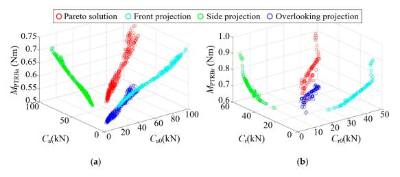
**Figure 7.** Axial and radial performance optimization results of PTRB. (**a**) Axial performance optimization results. (**b**) Radial performance optimization results.
