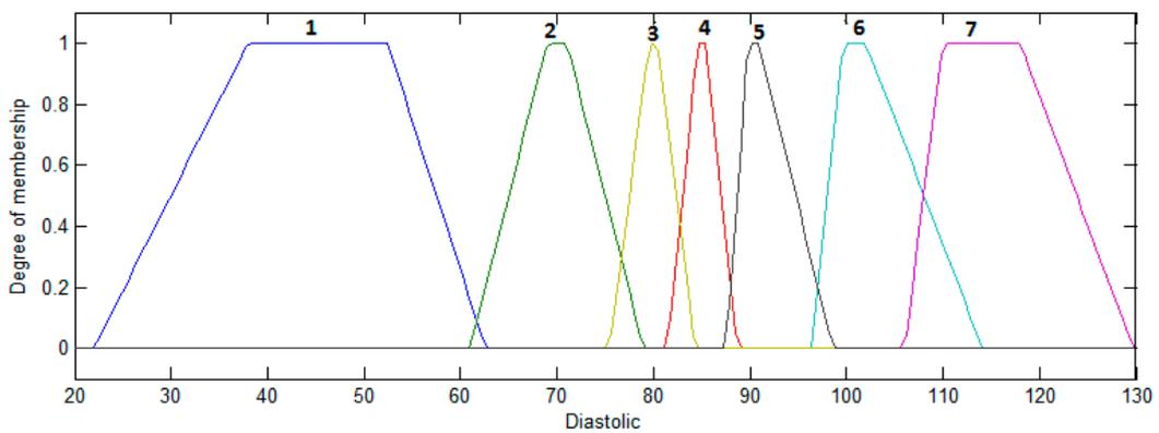
**Figure 5.** Diastolic input for the type-1 FS for classification with trapezoidal membership functions.
