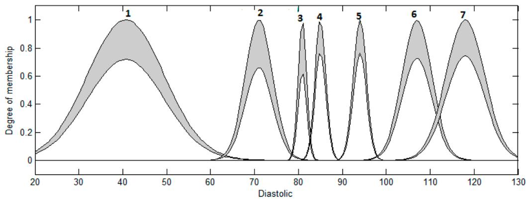
**Figure 46.** Diastolic input for the optimized interval type-2 fuzzy system for classification with Gaussian membership functions.
