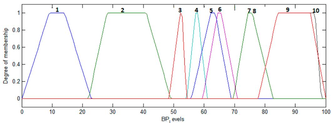
**Figure 6.** BP\_Levels output for the type-1 FS for classification with trapezoidal membership functions.
