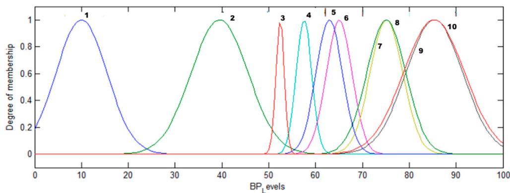
Figure 15. BP\_Levels output for the type-1 fuzzy system for classification with Gaussian membership functions.
