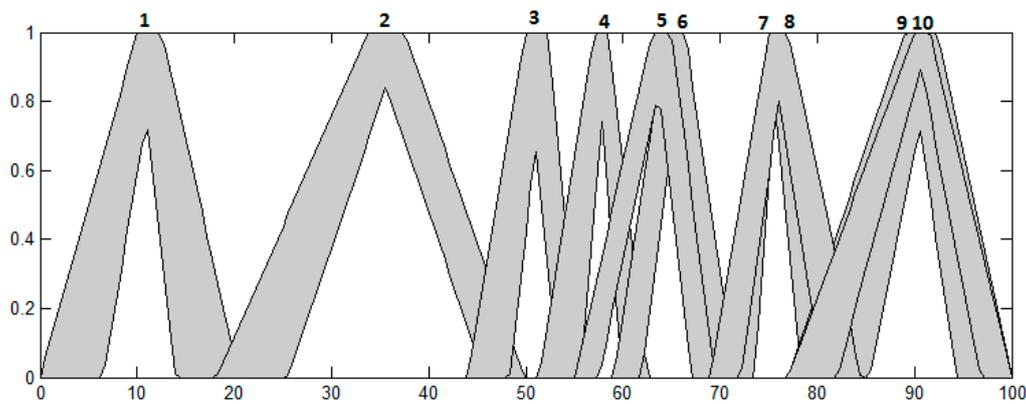
**Figure 24.** BP\_Levels output for the interval type-2 FS for classification with triangular membership functions.
