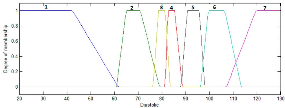
**Figure 10.** Diastolic input for the optimized type-1 FS for classification with trapezoidal membership functions.
