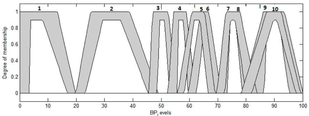
**Figure 38.** BP\_Levels output for the optimized interval type-2 fuzzy system for classification with trapezoidal membership functions.
