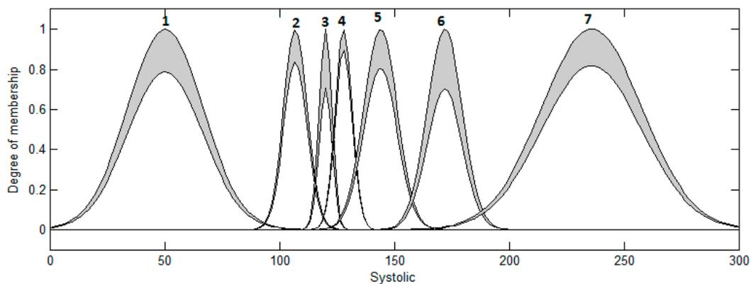
**Figure 40.** Systolic input for the interval type-2 fuzzy system for classification with Gaussian membership functions.
