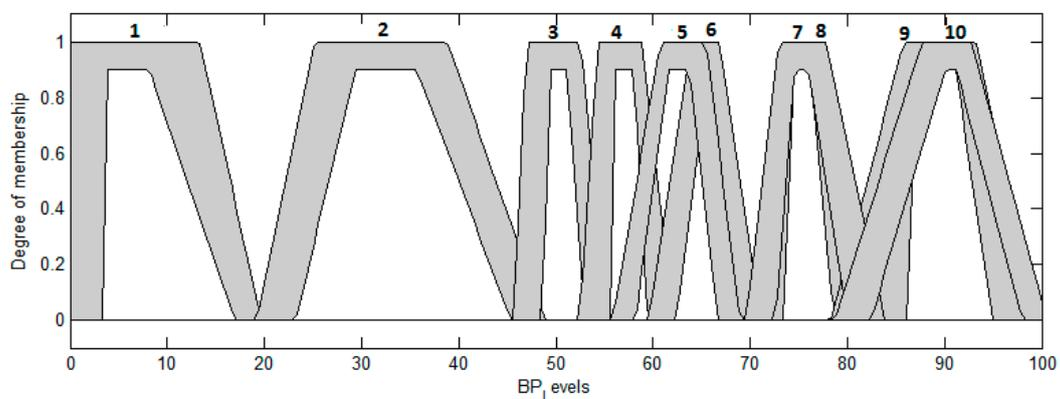
**Figure 33.** BP\_Levels output for the interval type-2 fuzzy system for classification with trapezoidal membership functions.
