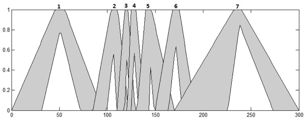
Figure 22. Systolic input for the interval type-2 FS for classification with triangular membership functions.
