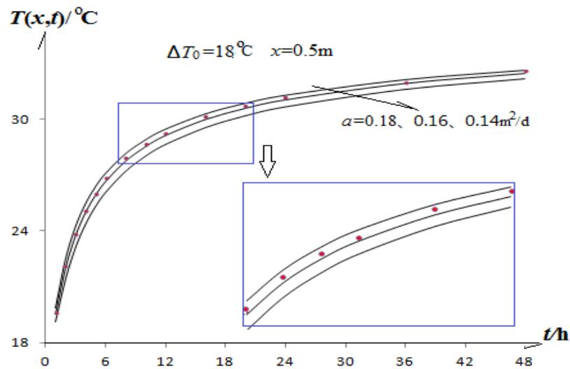
**Figure 5.**  $T(x,t) - t$  curve fitting method for  $a$ .
