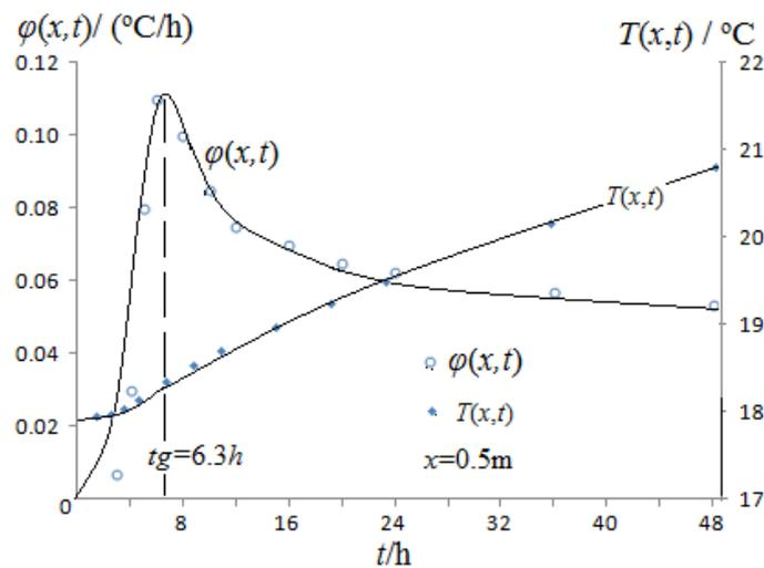
Figure 4. The inflection point method for finding  $a$ .
