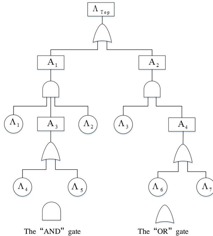
Figure 1. A fault tree structure.
