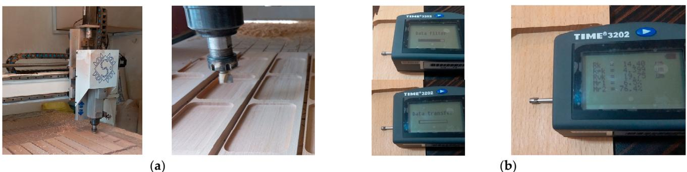
**Figure 1.** (a) CNC machining of beech wood; (b) surface roughness measurement.
