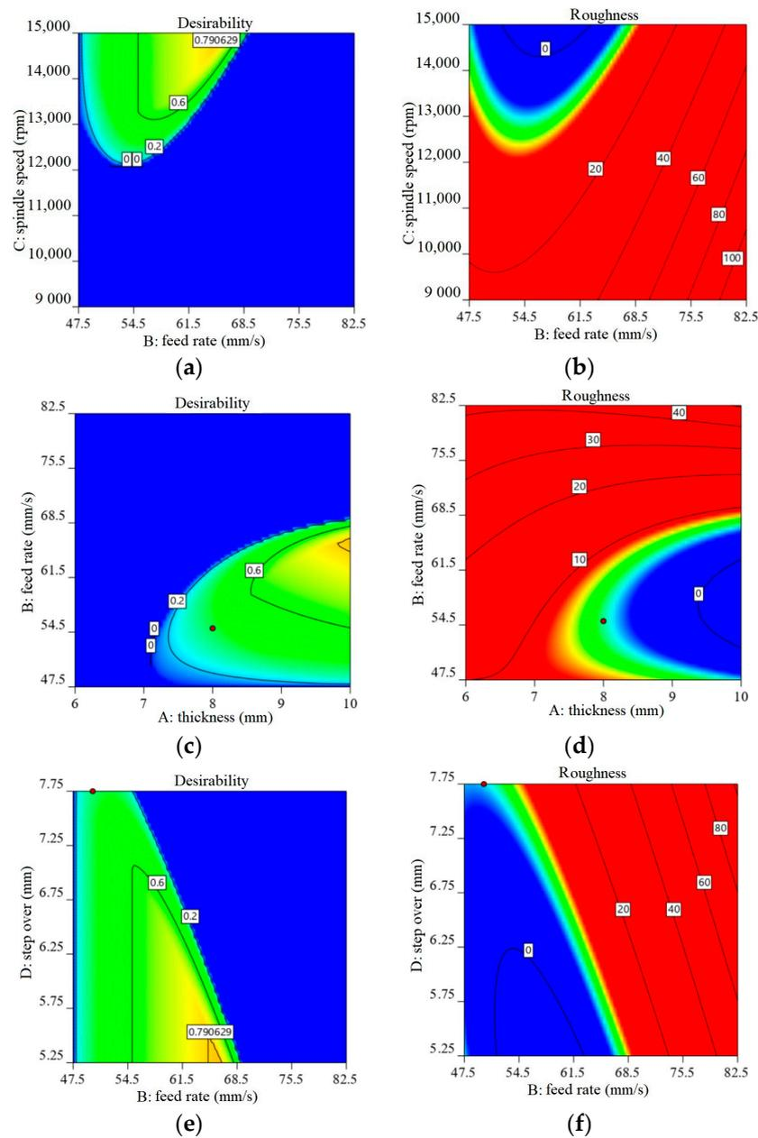
**Figure 3.** Effect of machining parameters and graphical analysis for surface roughness and desirability: (a) spindle speed and feed rate on desirability; (b) spindle speed and feed rate on roughness; (c) feed rate and thickness on desirability; (d) feed rate and thickness on roughness; (e) feed rate and step over on desirability; (f) feed rate and step over on roughness.
