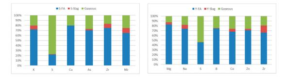
Figure 8. Partitioning for some volatile elements at ESP at Shenhuo (left) and Yihua (right) power plants.
