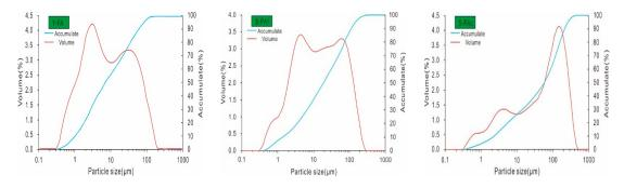
**Figure 4.** Particle-size distribution of Y-FA, S-FAf, and S-FAc. Y-FA, fly ash from Yihua power plant; S-FAf and S-FAc, fine fly ash and coarse fly ash from Shenhuo power plant.
