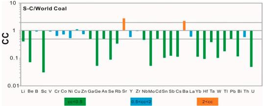
**Figure 3.** Concentration coefficients of trace elements in feed coal from Shenhuo power plant normalized to corresponding average values in Chinese [50] and worldwide [51] coals (modified after Dai et al., 2015) [29].
