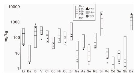
**Figure 6.** Concentrations of selected trace elements in the fly ashes at Shenhuo and Yihua power plants compared with the corresponding maximum, minimum, P25, P50, and P75 values in European fly ashes [52].
