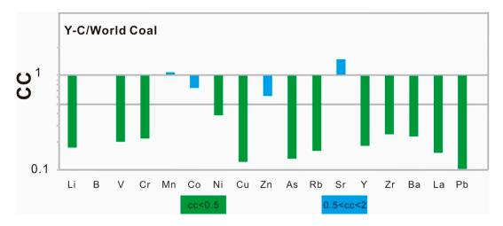
**Figure 2.** Concentration coefficients of trace elements in feed coal from Yihua power plant normalized to average values in Chinese [50] and worldwide [51] coals (modified after Dai et al., 2015) [29].
