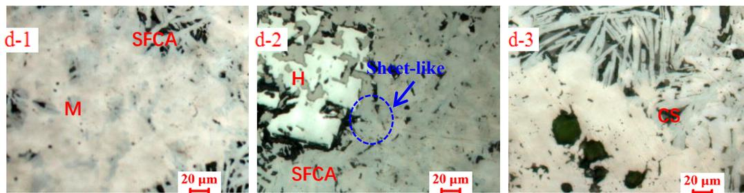
**Figure 5.** Effects of  $\text{Al}_2\text{O}_3$  content on microstructure. (a-1,a-2,a-3)  $\text{Al}_2\text{O}_3 = 1.00\%$ ; (b-1,b-2,b-3)  $\text{Al}_2\text{O}_3 = 1.55\%$ ; (c-1,c-2,c-3)  $\text{Al}_2\text{O}_3 = 1.80\%$ ; (d-1,d-2,d-3)  $\text{Al}_2\text{O}_3 = 2.25\%$ ; M—magnetite; H—hematite; CS—silicate.
