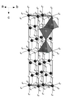
**Figure 2.** The crystal structure of spiridonovite. *M* (Cu,Ag) sites and Te atoms are given as white and black circles, respectively. The tetrahedral coordination of the *M* sites is shown as isolated polyhedra. The unit cell and the orientation of the structure are outlined.
