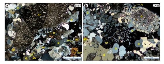
**Figure 10.** (a) Micrographic intergrowths of quartz and myrmekite develop around the alkali feldspar from the ZK57; (b) The alkali feldspar was replaced by the quartz from the ZK65. Q–quartz, Kf–feldspar, Bt–biotite, Ms–muscovite, Pl–plagioclase; Hbl–hornblende.
