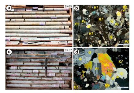
**Figure 3.** Drill cores and micrographics of ZK65 and ZK57 from the Xinfeng mine, Xianghualing area, South China. (**a**,**b**) Biotite monzonitic granites from ZK65. (**c**,**d**) Two-mica monzonitic granite from ZK57. Q, quartz; Kf, feldspar; Bt, biotite; Ms, muscovite; Pl, plagioclase.
