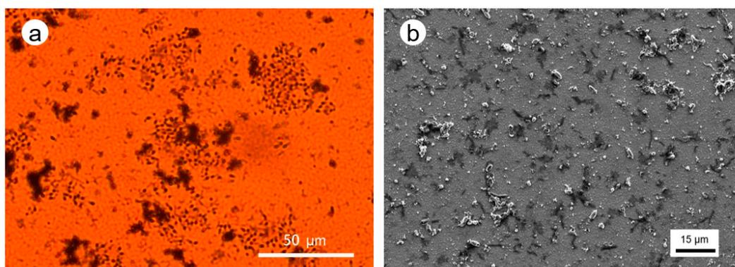
**Figure S1.** (a) Light microscopy picture of bio-photoanode; (b) ESEM picture of bio-photoanode.
