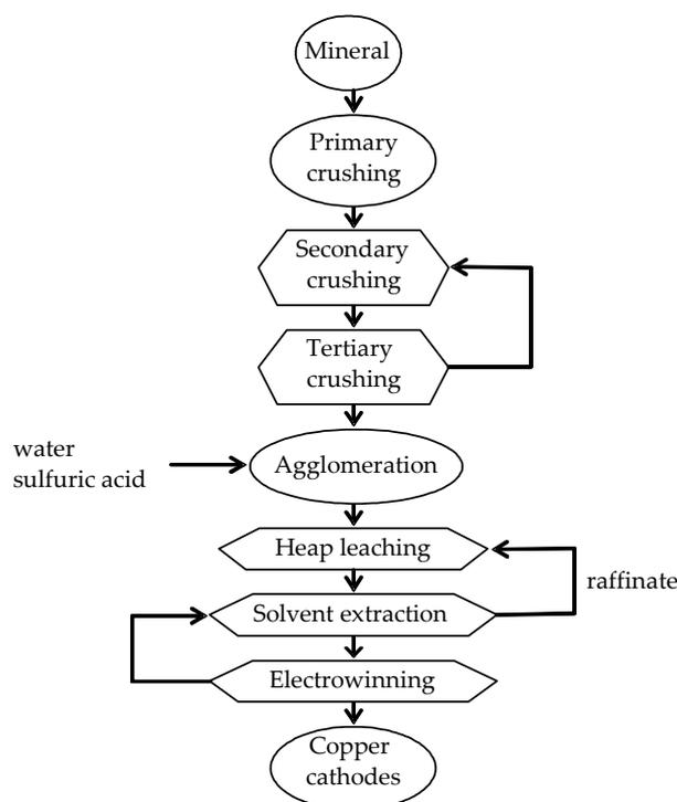
**Figure 1.** Block diagram of a copper heap bioleaching process [22].
