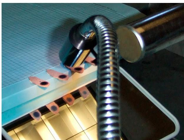
**Figure 3.** Experimental setup to permit simultaneous observation of ink applied to tops of slabs and image in mirror, angled below, of breakthrough ink on the undersides of slabs. Metal gooseneck piece in foreground is a high-intensity lamp.
