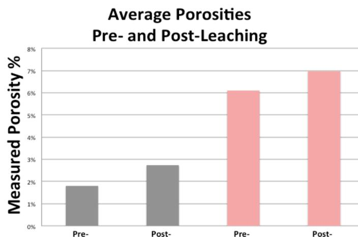
**Figure 6.** Average (15 samples per color) porosity pre- and post-leaching, showing an increase in porosity after sulfuric acid dissolution. Gray bars represent gray samples; red bars represent pink samples.
