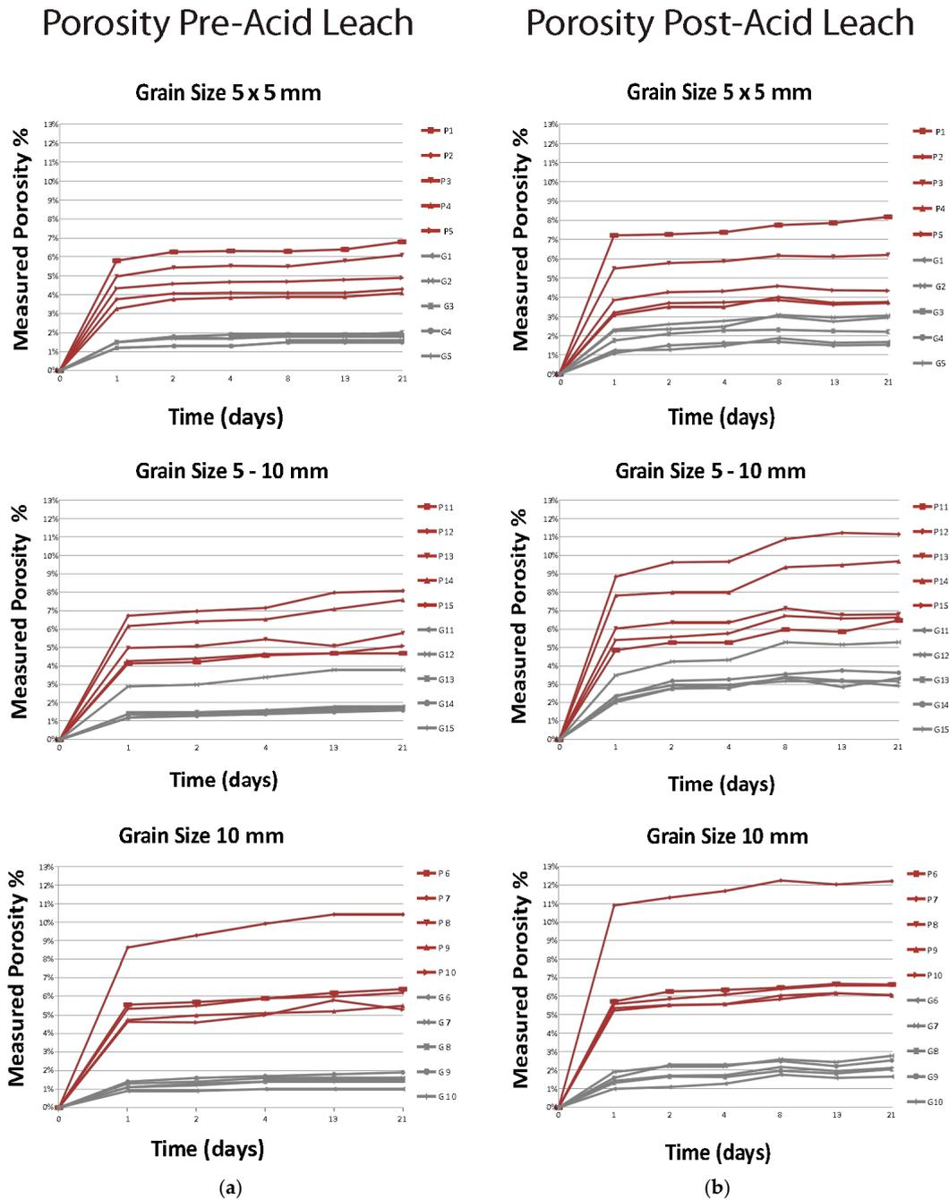
Figure 5. Estimated porosity measurements: (a) Pre-acid leach experiments; (b) Post-acid leach experiments. Red lines = pink samples; Gray lines = gray samples.
