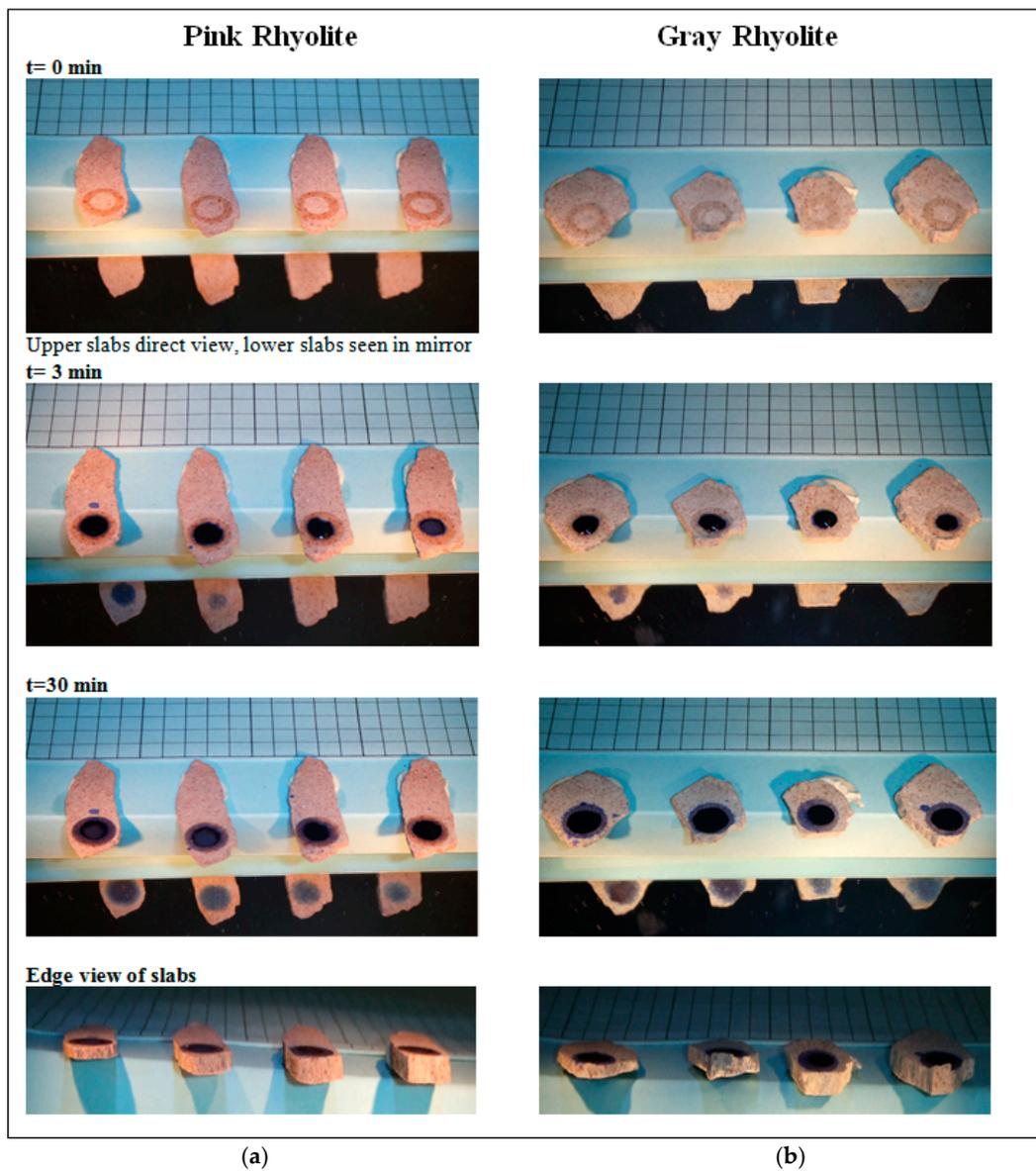
**Figure 7.** Timed ink penetration of rhyolite slabs to determine permeability. Boxes = 0.5 cm. (a) Pink rhyolite; (b) Gray rhyolite. Circles seen at  $t = 0$  are the ridges created by nail polish, which serve to contain and restrain the ink.
