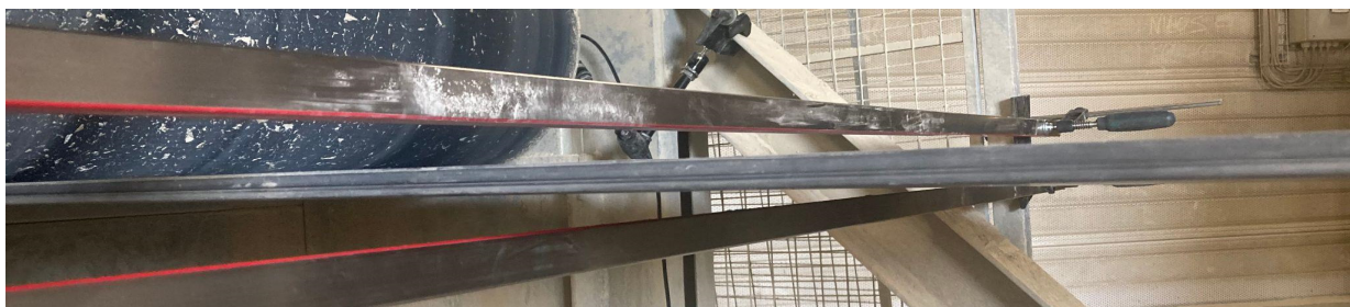
Figure 2. Installation of the magnetizing heads on the inspected conveyor belt.
