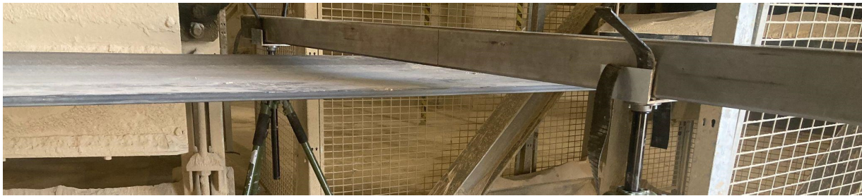
Figure 1. Installation of the measuring head on the inspected conveyor belt.
