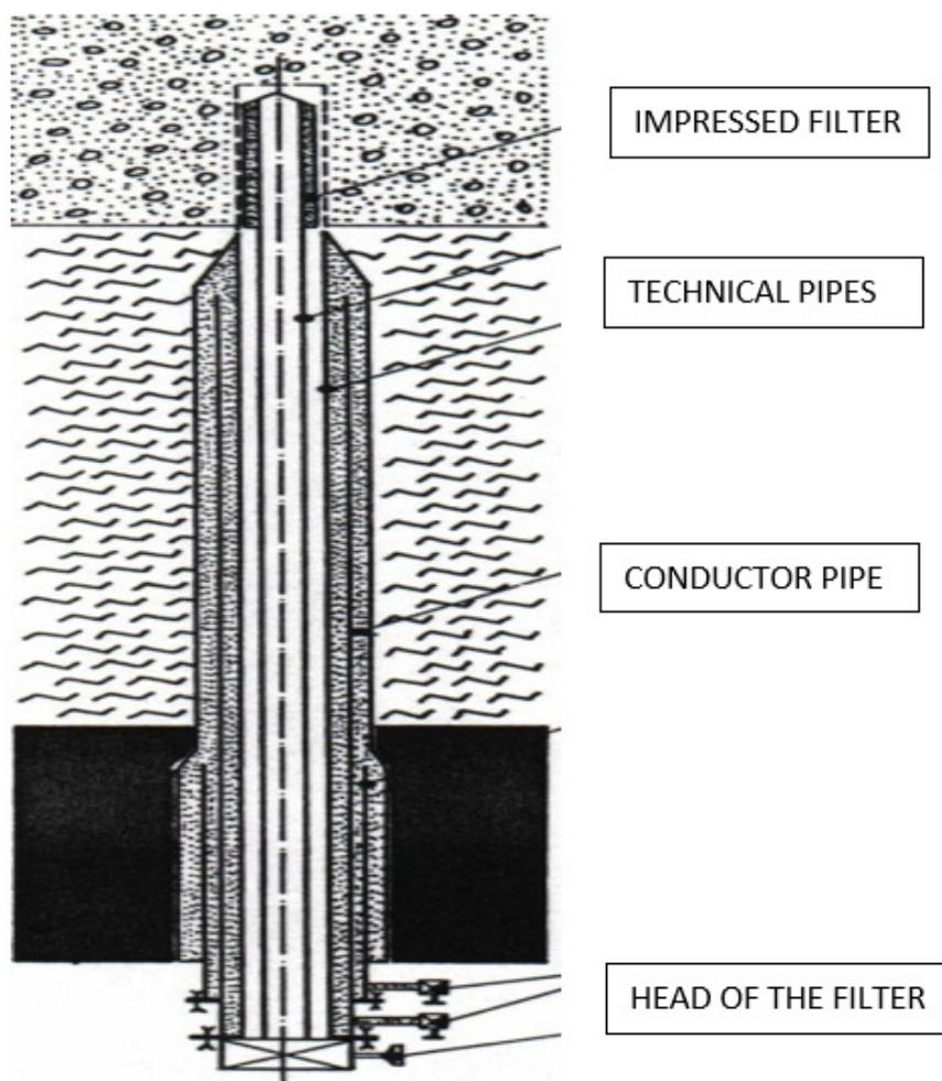
**Figure 6.** An impressed filter.
