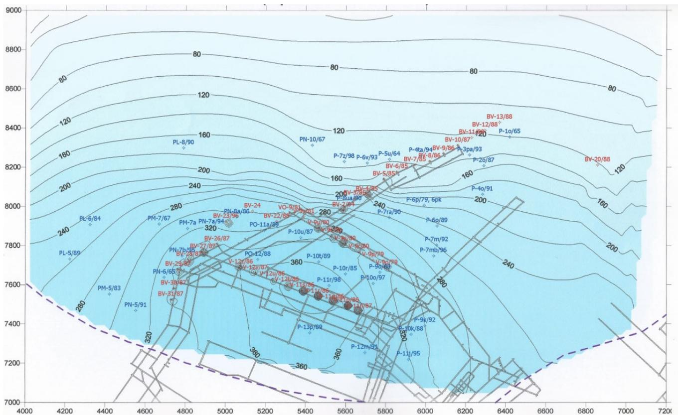
**Figure 4.** Calculated depressions in overburden aquifers.
