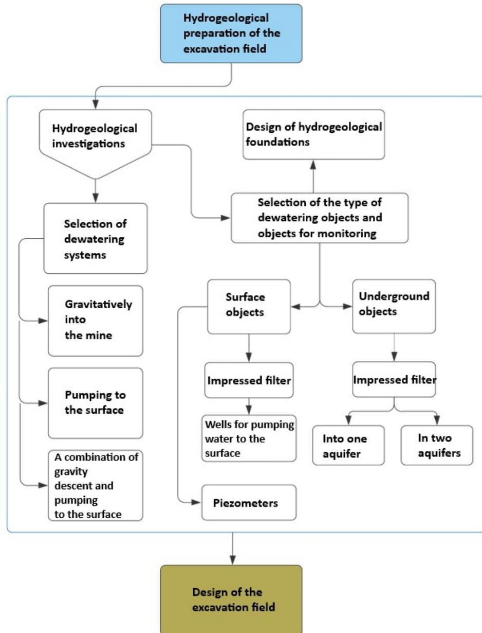
Figure 3. Hydrogeological activities for the design of a new excavation field.
