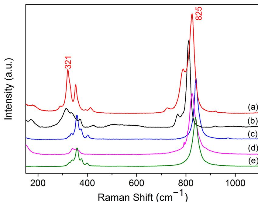
**Figure 3.** Raman spectra of mineral (a) vanadinite, (b) mimetite, (c) crocoite and synthetic pigments; (d) chrome yellow-orange and (e) chrome yellow deep.
