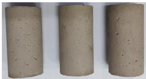
Figure 4. Cemented tailings backfill specimens.
