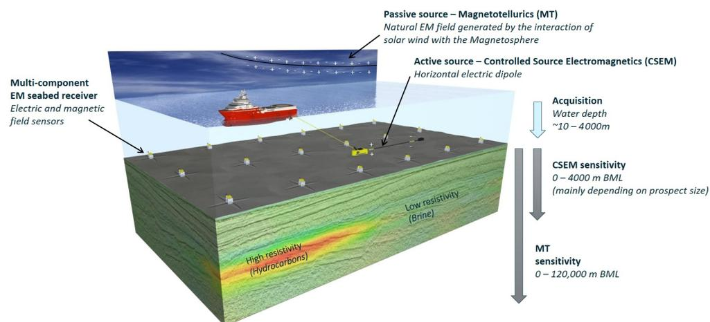
**Figure 1.** CSEM acquisition scheme and the state-of-art technology sensitivity below mud line (BLM) of the MT (up to 120 km depths) and CSEM (reservoirs up to 4 to 5 km burial) methods. Courtesy of EMGS.
