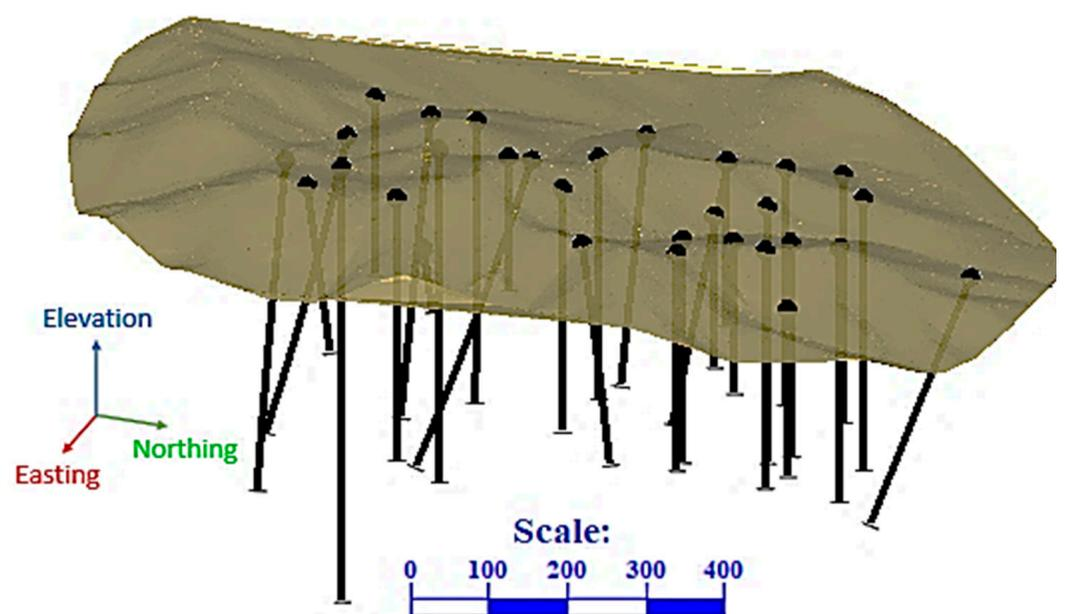
**Figure 3.** A 3D map of the drill holes (topography surface and boreholes are shown in brown and black, respectively).
