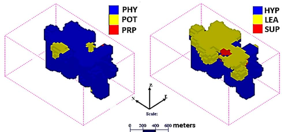
**Figure 2.** A block model of the Iju deposit showing alteration and mineralized zones.
