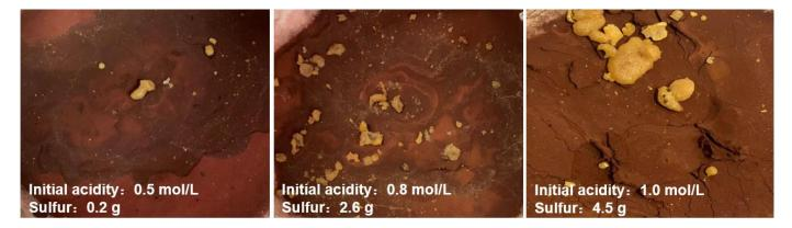
Figure 4. Images of the pressure leaching products with different initial acidity.
