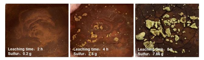
Figure 7. Images of the pressure leaching products with different leaching times.
