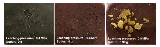
Figure 13. Images of the pressure leaching products at different oxygen pressure.
