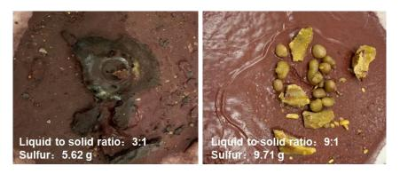
Figure 16. Images of the pressure leaching products with different liquid-to-solid ratios.
