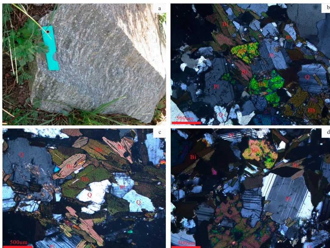
**Figure 3.** Field photograph and microphotographs of Yamusi granodiorite: (a) field photograph of Yamusi granodiorite; (b–d) microphotographs of Yamusi granodiorite. Abbreviations: Hb, amphiboles; Bi, biotite; Pl, plagioclase; and Q, quartz.
