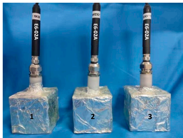
Figure 1. Internal relative humidity test specimen under sealed condition.
