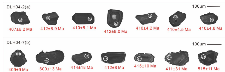
Figure 5. Cathodoluminescence (CL) images and zircon U-Pb ages from the felsic volcanic rocks of the Maoniushan Formation.
