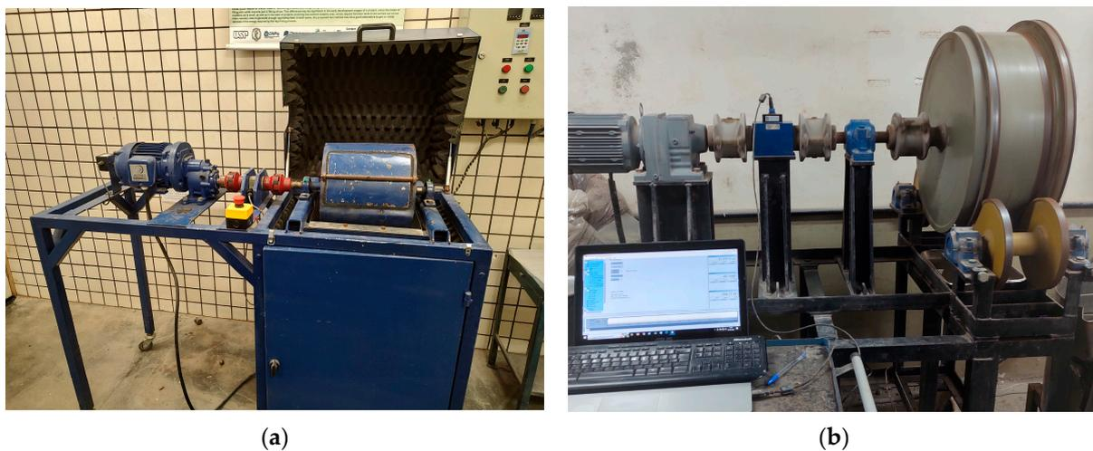
**Figure 2.** Test mills. (a) LTM-USP 305 mm × 305 mm mill; (b) LTM-UFRJ 580 mm × 240 mm mill.
