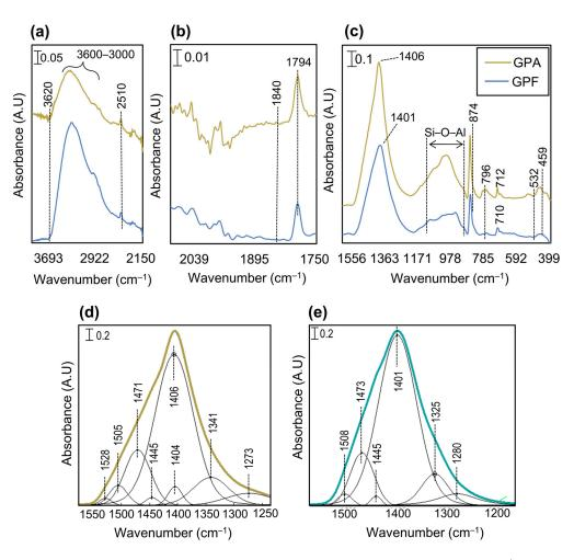
**Figure 6.** FTIR spectra of synthesized geopolymer composites: (a) 4000–2150 cm<sup>-1</sup>, (b) 2140–1750 cm<sup>-1</sup>, (c) 1600–400 cm<sup>-1</sup> and deconvoluted spectra between 1600 and 1200 cm<sup>-1</sup> for GPA (d) and GPF (e). Note that the black plots in (d,e) are deconvoluted peaks.
