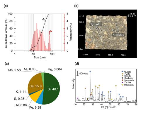
Figure 2. (a) Particle size distribution, (b) photomicrograph, (c) chemical composition and (d) XRD pattern of the ASGM tailings sample used in this study.
