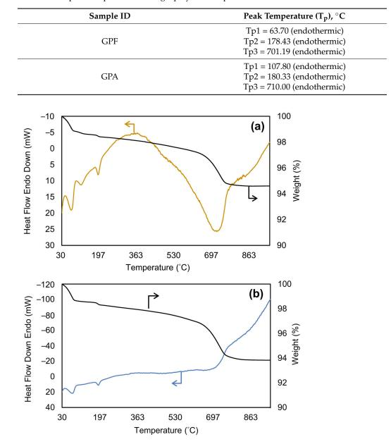
Table 3. DTA peak temperature of the geopolymer composites.
