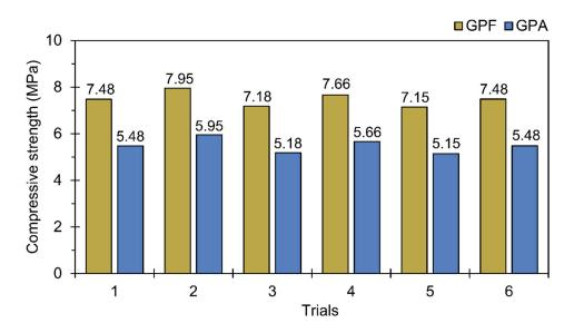
**Figure 9.** Unconfined compressive strengths (UCS) of geopolymer composites without POFA (GPA) and with POFA (GPF).
