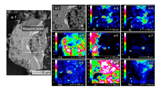
**Figure 7.** (**a-1**) Photomicrograph of GPA and (**a-2**) the mapped area with corresponding elemental maps of Al (**a-3**), Si (**a-4**), Ca (**a-5**), Fe (**a-6**), S (**a-7**), Mg (**a-8**), O (**a-9**) and Na (**a-10**).
