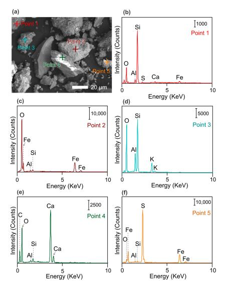
**Figure 3.** Photomicrograph of ASGM tailings (**a**) and the corresponding elemental point analysis of selected particles: Point 1 (**b**), Point 2 (**c**), Point 3 (**d**), Point 4 (**e**) and Point 5 (**f**). Note the differences in the scale of the *y*-axis of the EDS spectra.
