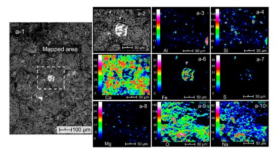
**Figure 8.** (**a-1**) Photomicrograph of GPF and (**a-2**) mapped area with corresponding elemental maps of Al (**a-3**), Si (**a-4**), Ca (**a-5**), Fe (**a-6**), S (**a-7**), Mg (**a-8**), O (**a-9**) and Na (**a-10**).
