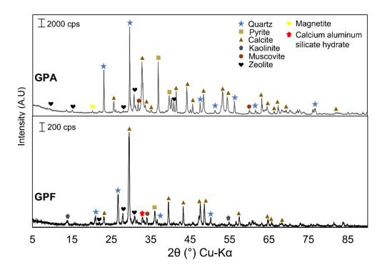
**Figure 5.** XRD patterns of synthesized geopolymer composites without POFA (GPA) and with POFA (GPF).
