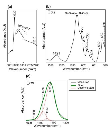
**Figure 4.** FTIR spectrum of the ASGM tailings sample: (a)  $4000-2400 \text{ cm}^{-1}$ , (b)  $1600-399 \text{ cm}^{-1}$ , and (c) deconvoluted spectrum between 1650 and 1250 cm<sup>-1</sup>.
