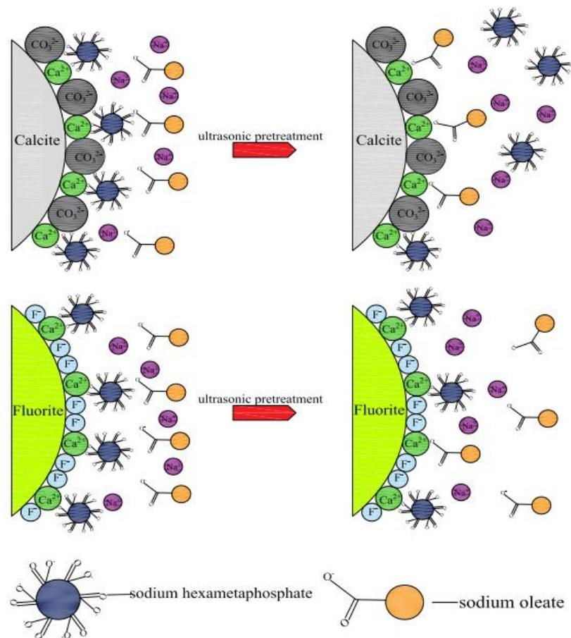
**Figure 14.** Mechanism model of ultrasonic pretreatment.
