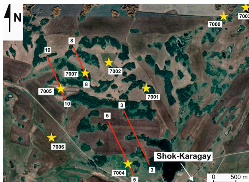
**Figure 2.** Location of exploration wells (points 7001–7007) overlaid on a geological map of the Shok-Karagay deposit. Scale: 1:25,000. Schemes follow the same formatting (Google Maps) [23]. Red lines: cross-sections. Yellow stars: sampling points.
