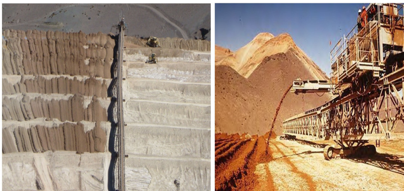
Figure 12. Practical experience using mobile stacking conveyor with tripper car for disposal of filtered mine tailings in La Coipa Mine, Chile [30].
