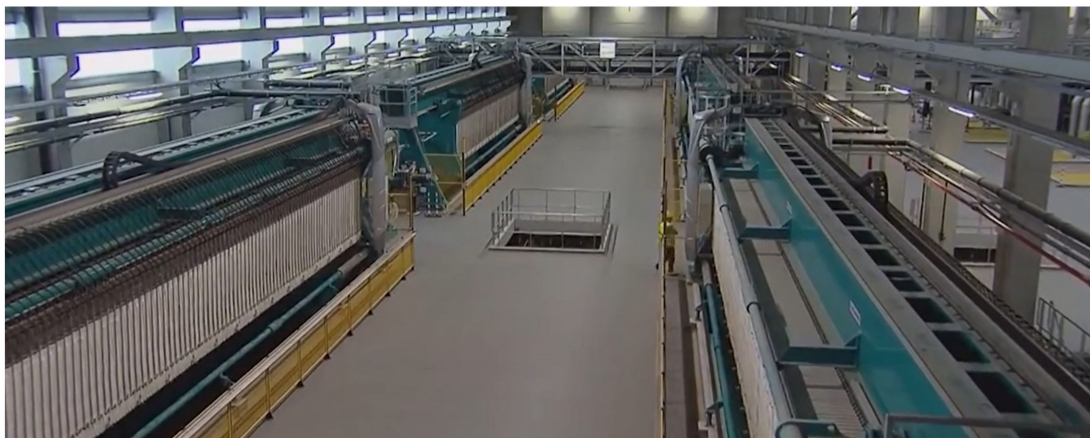
Figure 6. Example of mine tailings filtering plant with use of filter presses.
