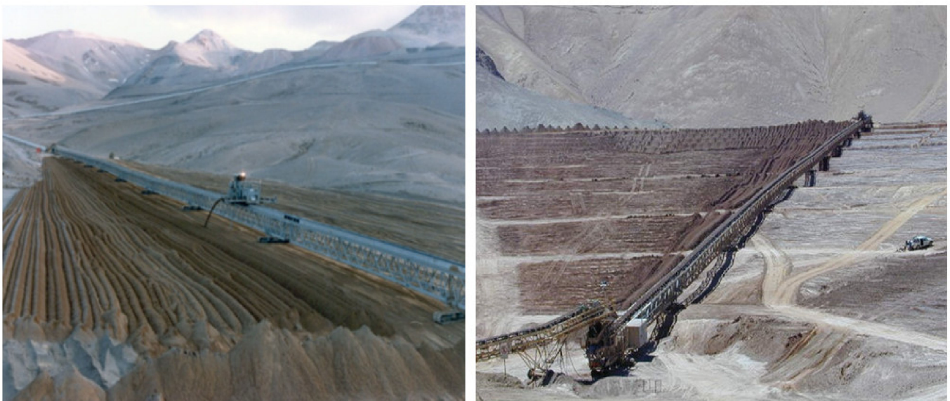
Figure 14. Example of filtered mine tailings disposal considering abrupt topography in La Coipa Mine, Chile [30].
