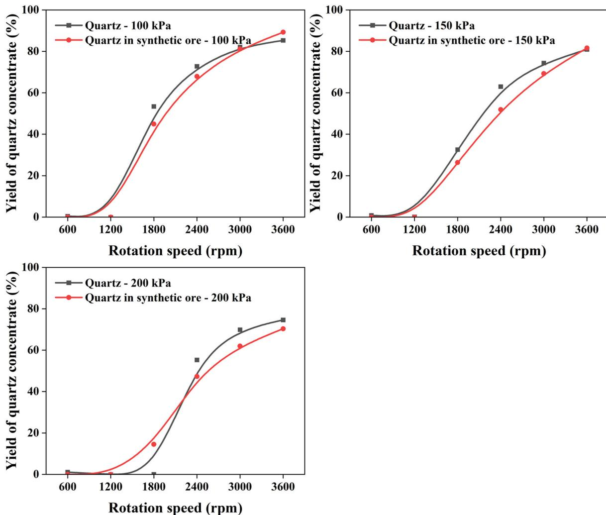
**Figure 9.** The yield in the quartz concentrate with single quartz and synthetic ore tests.
