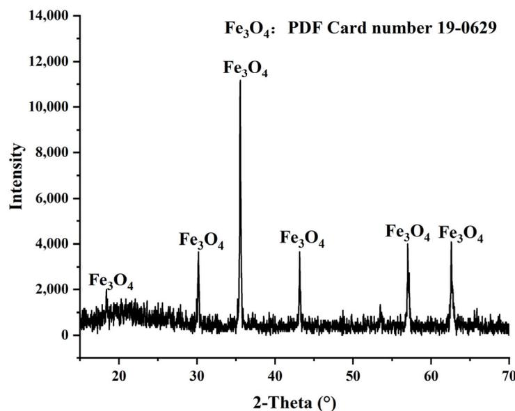
Figure 3. The XRD pattern of magnetite.
