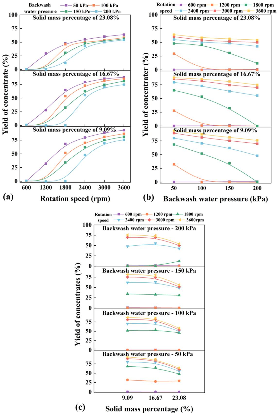
Figure 5. Yield of concentrate as a function of rotation speed (a), backwash water pressure (b), and solid mass percentage (c).
