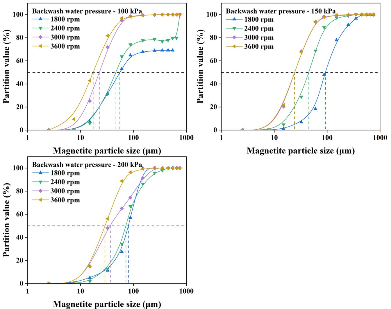
Figure 12. The magnetite partition curves in the synthetic ore classification tests at 16.67% solid mass percentage of feed.
