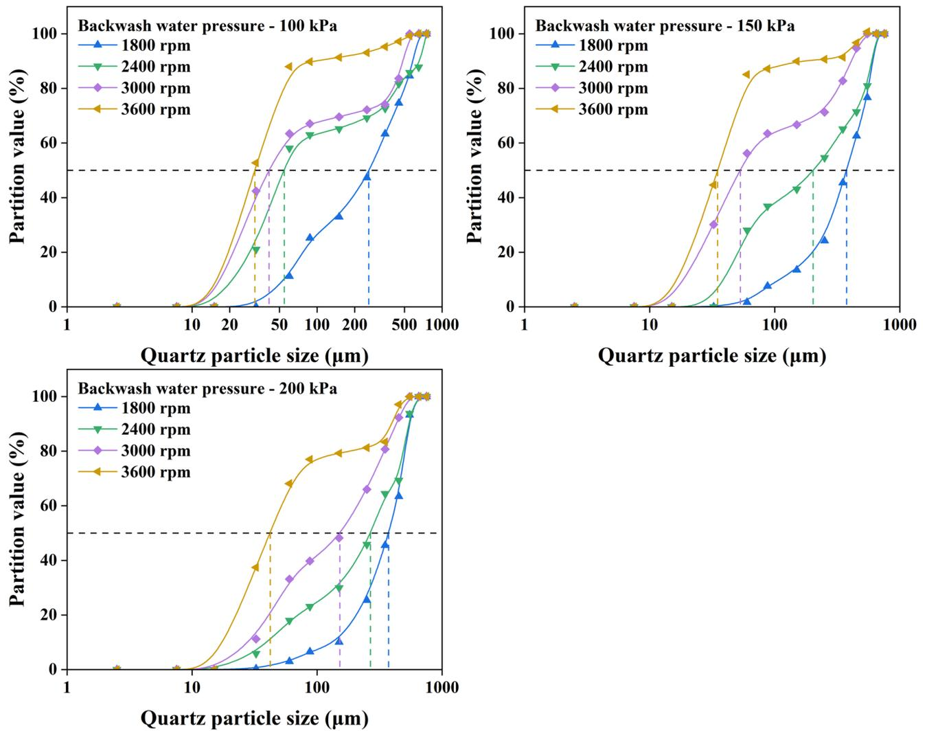
Figure 11. The quartz partition curves in the synthetic ore classification tests at 16.67% solid mass percentage of feed.
