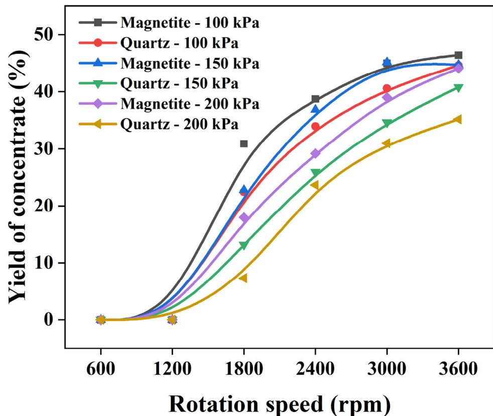
Figure 10. The yield of magnetite concentrate at different backwash water pressures.
