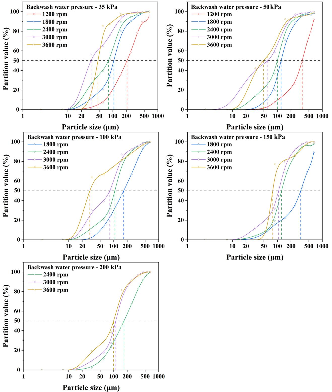
Figure 6. The partition curves of quartz at different rotation speeds and 16.67% solid mass percentage.
