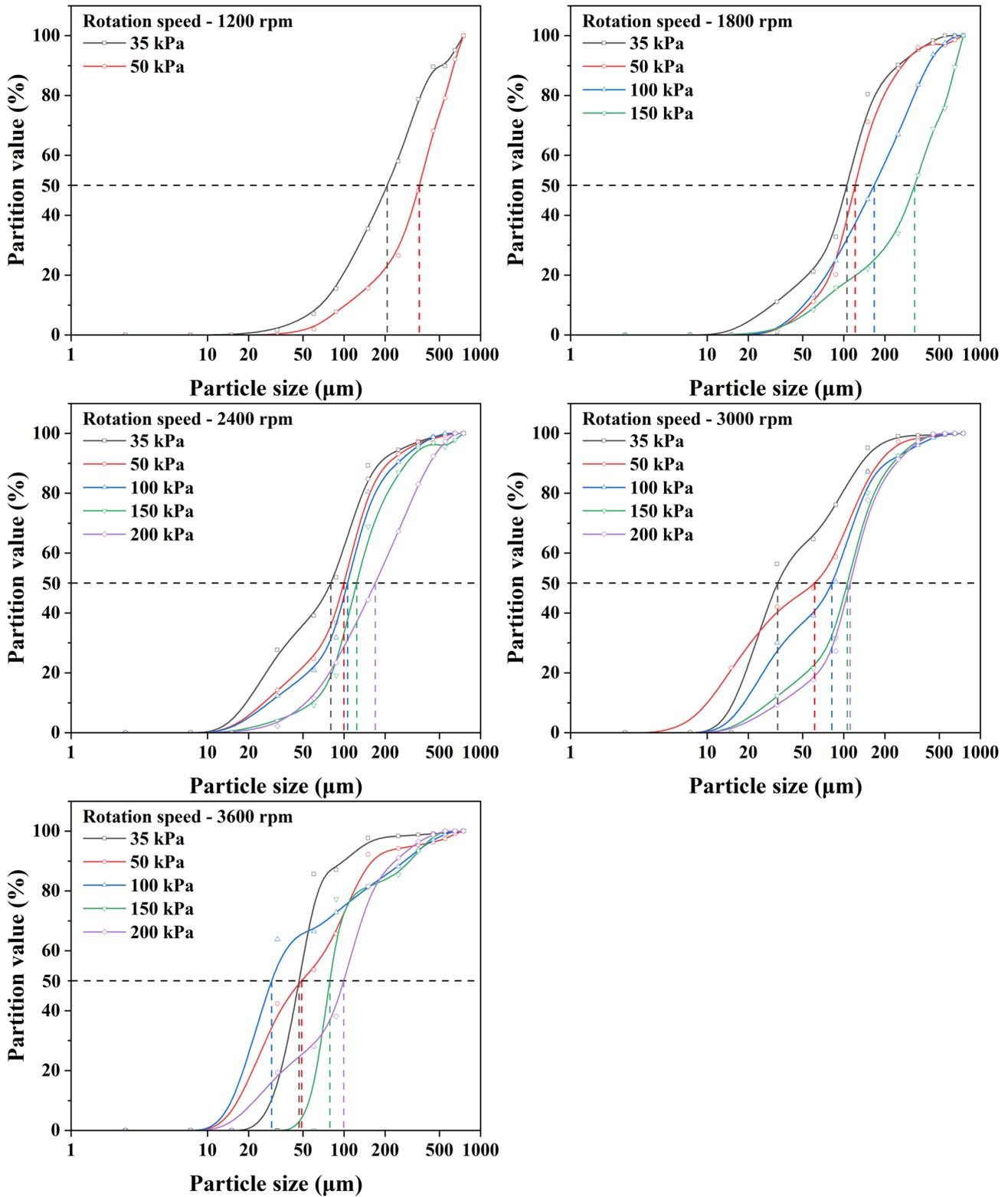
Figure 7. The partition curves of quartz at different backwash water pressures and 16.67% solid mass percentage.
