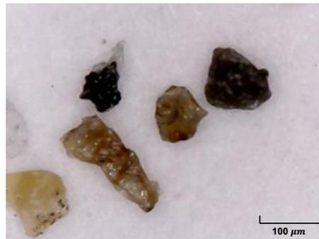
**Figure 10.** A stereo-microscope image of middling particles from a fine shaking table in a Turkish chromite beneficiation plant at 180 + 125  $\mu\text{m}$  size fraction [107].
