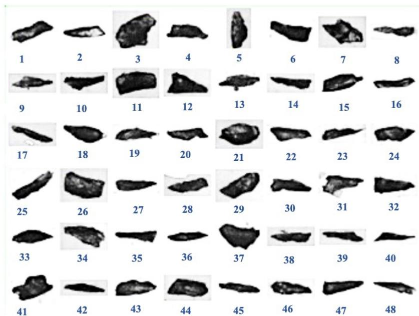
**Figure 18.** DIA images of ball-milled quartz particles.
