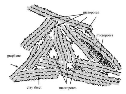
structures with interesting properties [24–26]. A possible structure of a representative clay carbon composite is shown in Figure 1 below.
