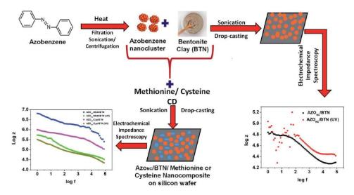
**Figure 4.** Protocol adopted to develop a photoresponsive carbon-dot-incorporated azobenzene nanocluster–clay (bentonite) hybrid with tunable conductivity (reproduced from ref. [64]; copyright 2020 Royal Society of Chemistry).
