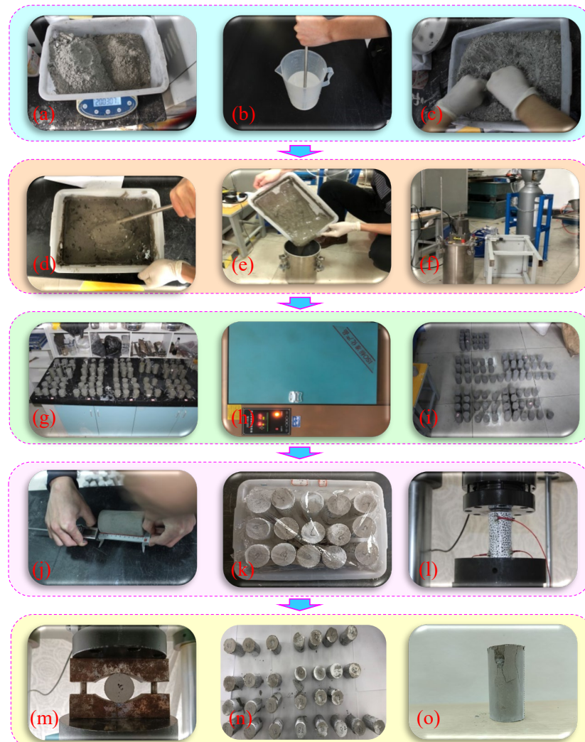
Figure 3. The process of preparing the CMFB specimens and the mechanical tests. (a–c): weighing and mixing of aggregate and auxiliary materials (d–f): development of fresh slurry of CMFB. (g–o): dimension calibration and mechanical test of CMFB samples.
