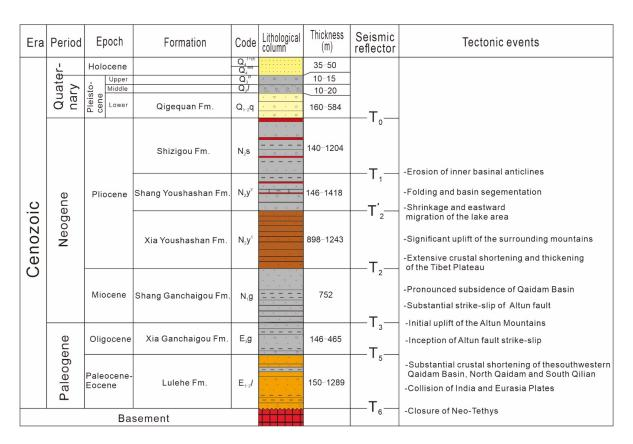
**Figure 3.** Cenozoic stratigraphical framework and seismic reflectors of the southwestern area of the Qaidam Basin (modified after [69,71,72]). Detailed regional tectonic events see [9].
