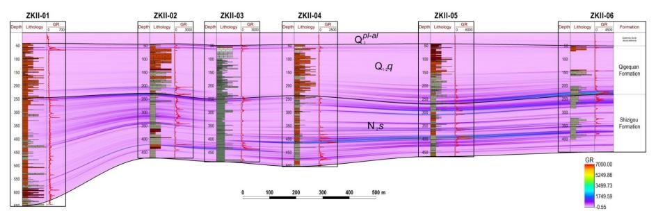
**Figure 4.** The well-tie profile to illustrate uranium ore horizons among industrial sandstone-hosted uranium boreholes in the Yuejin-II area (the contour-filled color was based on the Natural Gamma Logging Values (GR), with high values representing the uranium horizons).  $Q_3^{pl-al}$ -Quaternary pluvial-alluvial sediments,  $Q_{1-2}q$ -Quaternary Qigequan Formation,  $N_2$ s-Neogene Shizigou Formation.
