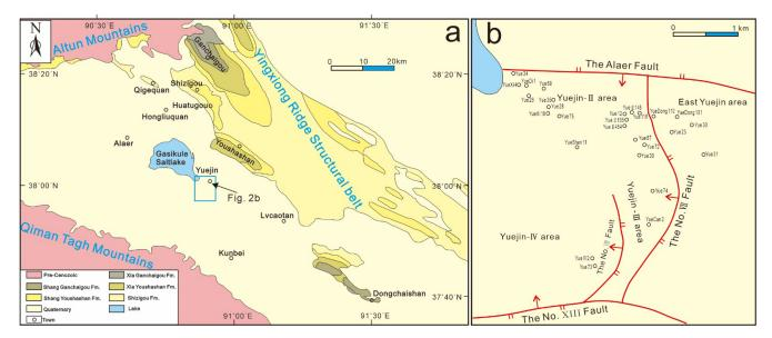
Figure 2. (a) Regional geological sketch of southwestern area of the Qaidam Basin and its adjacent orogenic areas (modified after [69]) and (b) schematic geological map of the Yuejin area to the main controlled faults and representative oilfield holes (modified after [70]).
