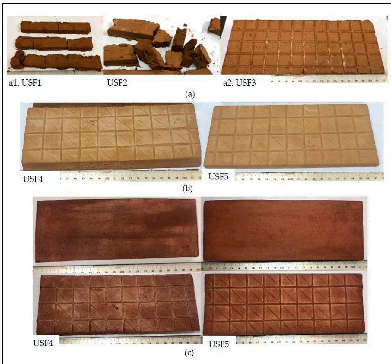
**Figure 7.** Tiles from NMW slip. (a) Failed casting using USF1, USF2 and USF3; (b) successful casting of tiles using USF4 and USF5; and (c) USF4 and USF5 tiles fired at 1050 °C.
