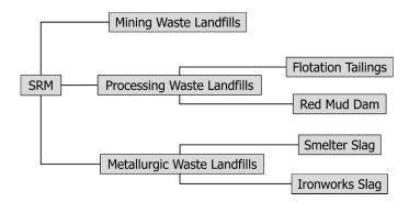
Figure 2. Types of mining, processing, and metallurgic waste.
