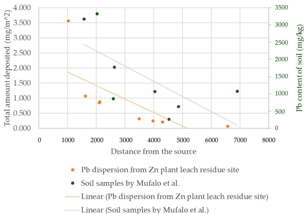
**Figure 8.** Comparison between simulated results of dispersion of Pb-bearing Zn plant leach residues and measured Pb content of soils by Mufalo et al. [10]: orange dots show Pb dispersion with consideration of water condition on the surface of the source by MNDWI; and green dots show measured Pb content of soils by Mufalo et al. [10].
