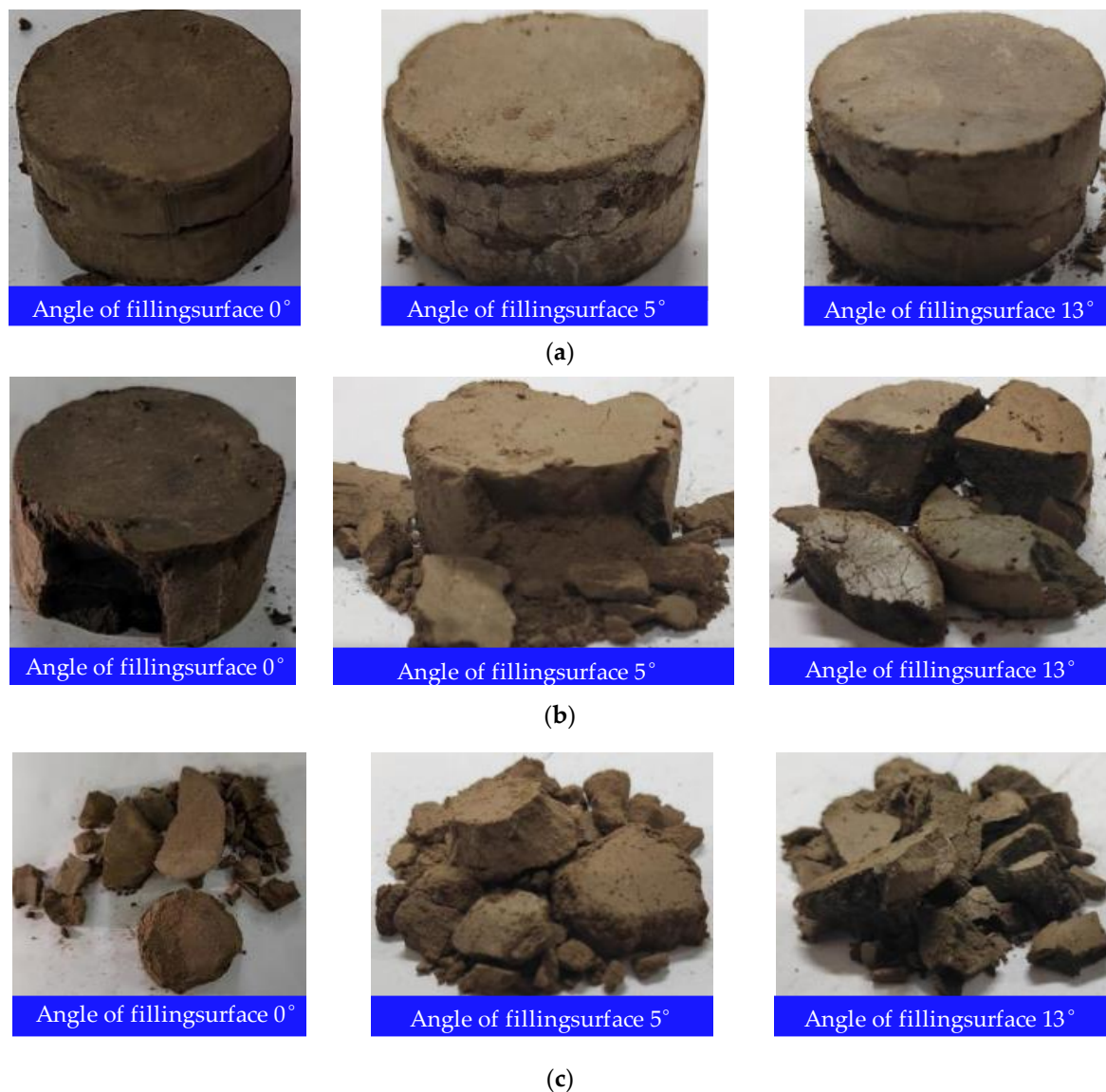
Figure 14. Influence of different filling surface angles on the failure mode of a layered filling body: (a) failure mode of layered filling body with approximate strain rate of 16 \text{ s}^{-1} ; (b) failure mode of layered filling body with approximate strain rate of 27 \text{ s}^{-1} ; (c) failure mode of layered filling body with approximate strain rate of 40 \text{ s}^{-1} .
