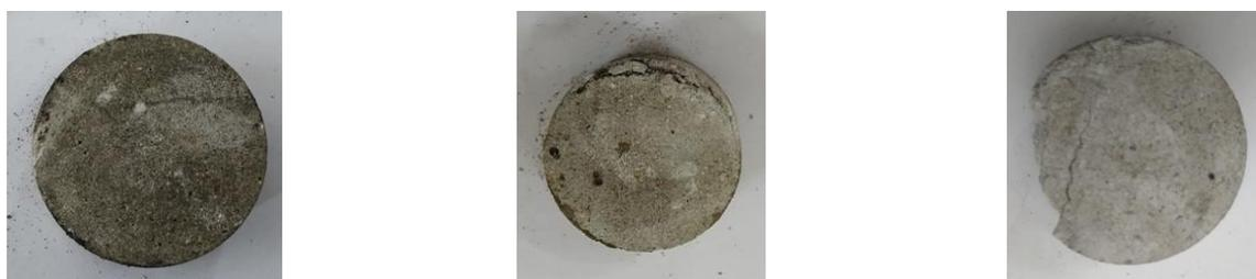
(a) 2 MPa confining pressure 0.2 impact (b) 2 MPa confining pressure 0.3 impact (c) 2 MPa confining pressure 0.4 impact (1)
