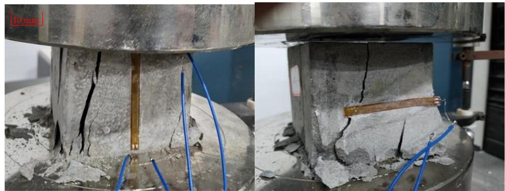
**Figure 2.** Static compressive strength and Poisson's ratio of similar materials were tested.
