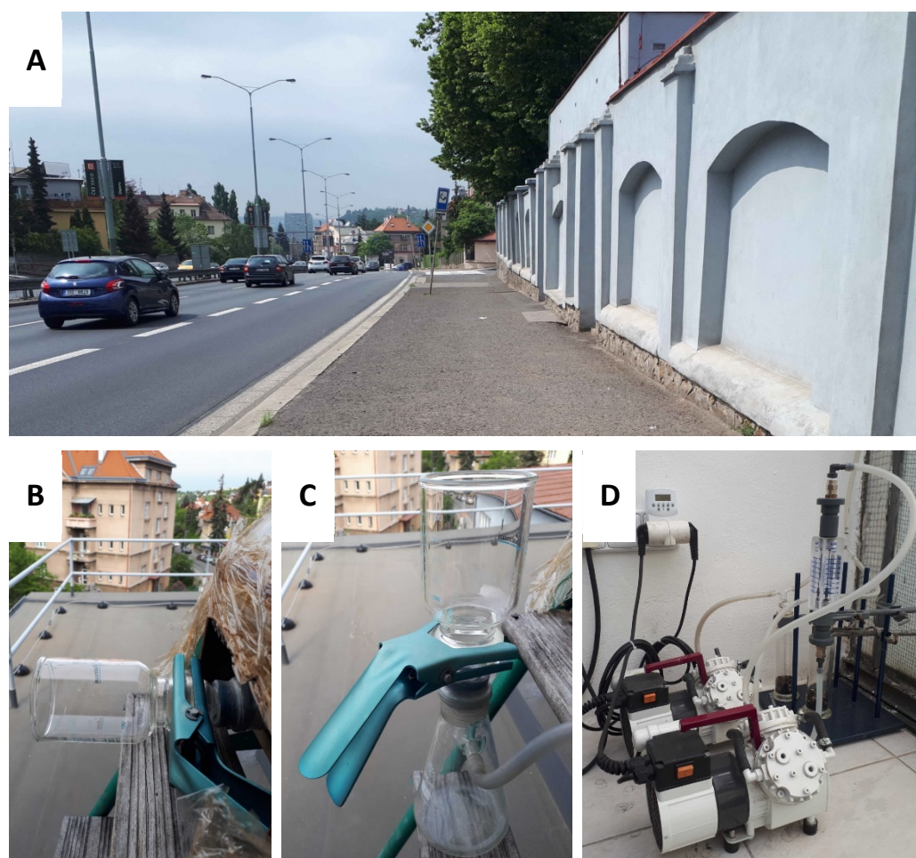
Figure 4. Sampling sites in the vicinity of the V Holešovičkách street. (A) Sampling stage 12/12–09/13, samples swept from wall surface (white ledge) at the street edge. (B,C) A setup used in sampling stages 06–07/14 and 02/15–04/16 positioned 50 m from the street at 10 m height, samples on filters. (D) Vacuum pump with airflow control (10 L/min).
