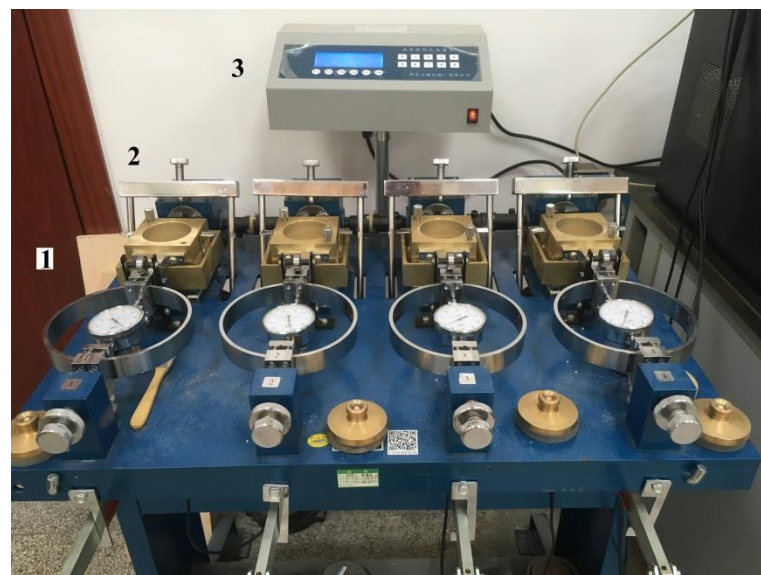
Figure 1. Equipment for direct shear test (DSJ-3). 1: strain meter; 2: shear box; 3: control panel.
