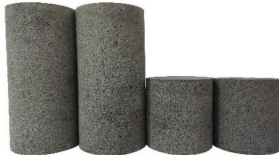
Figure 2. Coal measures sandstone specimens.
