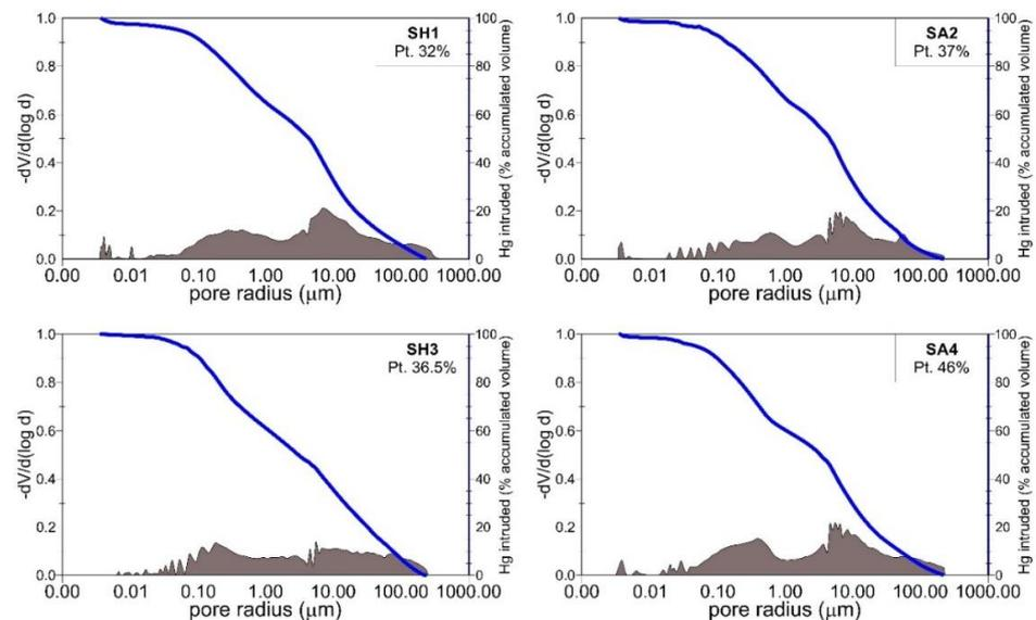
**Figure 6.** Porosimetric values of the samples studied. The relative volume of intruded Hg is shown in brown. The blue path represents the accumulated volume of intruded Hg (Pt = total porosity).
