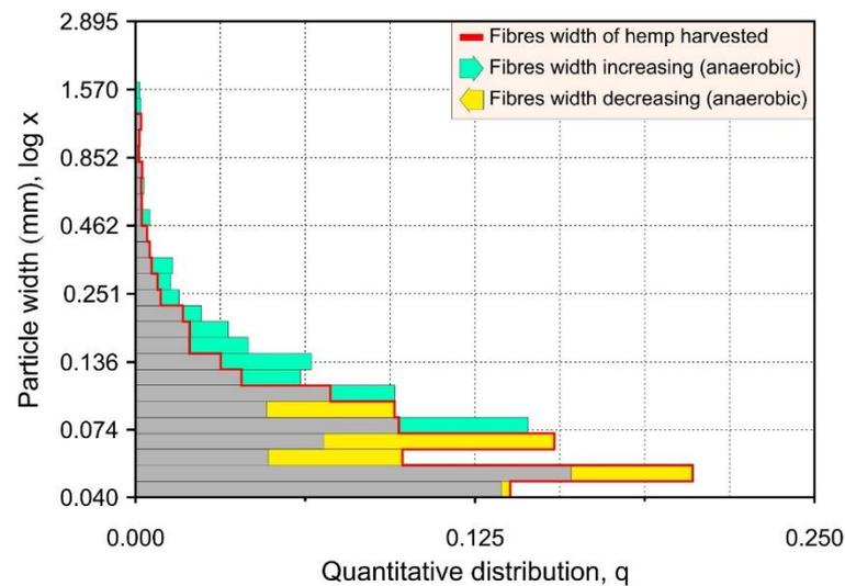
**Figure 1.** Width and quantitative distribution of the hemp fibres, using FiberShape.
