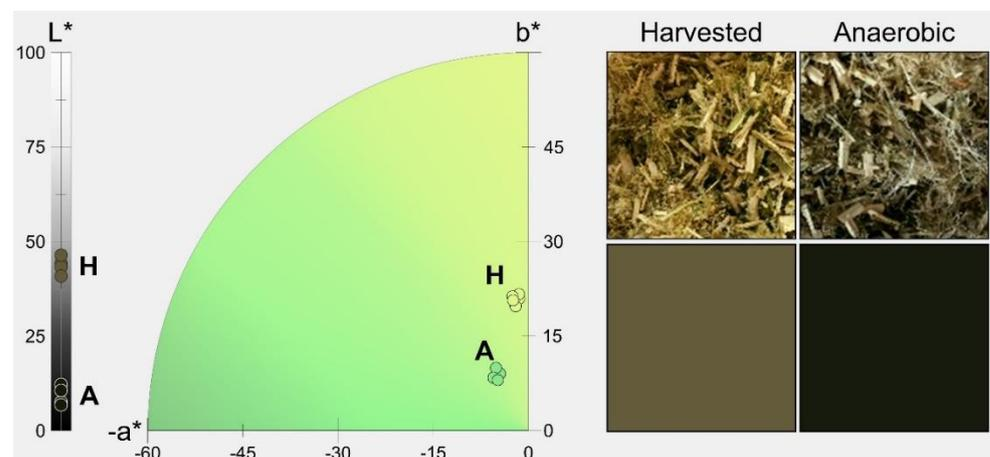
**Figure 2.** Visual comparison of the two types of hemp (freshly harvested and wet-anaerobic), and their colour representation according to CIELab1976 scheme [109].
