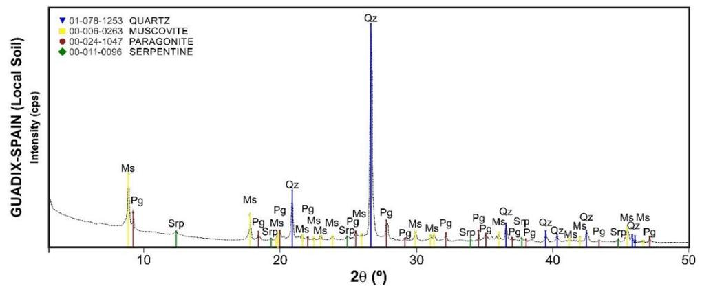
**Figure 3.** X-ray diffractogram for the clay. Legend: Qz = quartz; Pg = paragonite; Srp = serpentine; Ms = muscovite.
