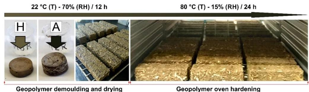
**Figure 4.** Demoulding, drying, and curing of the geopolymer concrete samples in an oven.
