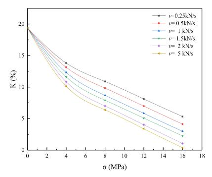
Figure 4. Porosity-stress curves of gangue specimens.
