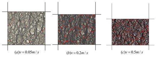
**Figure 12.** Fracture evolution of gangue models with different loading rates under the axial pressure of 4 MPa.
