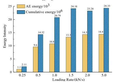
Figure 6. Histogram of AE energy-cumulative energy of gangue.
