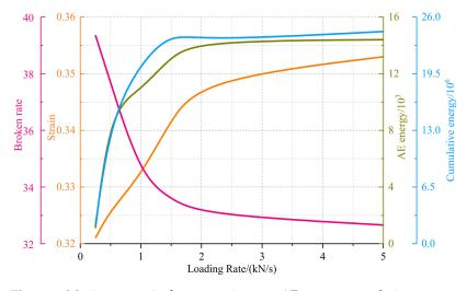
Figure 7. Maximum strain-fragmentation rate-AE energy-cumulative energy curve.
