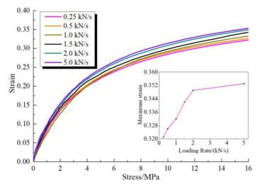
Figure 3. Stress-strain curve of gangue specimens at different loading rates under the confined compression.
