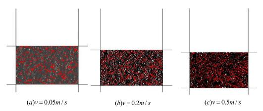
**Figure 13.** Fracture evolution of gangue models with different loading rates under the axial pressure of 16 MPa.
