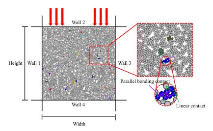
Figure 2. Backfilling of graded particle profiles.
